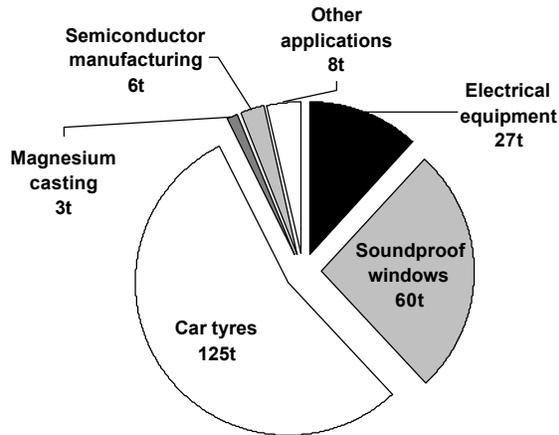
Figure 1: SF<sub>6</sub> emissions from different emission sources in Germany in 1998 (in t)
