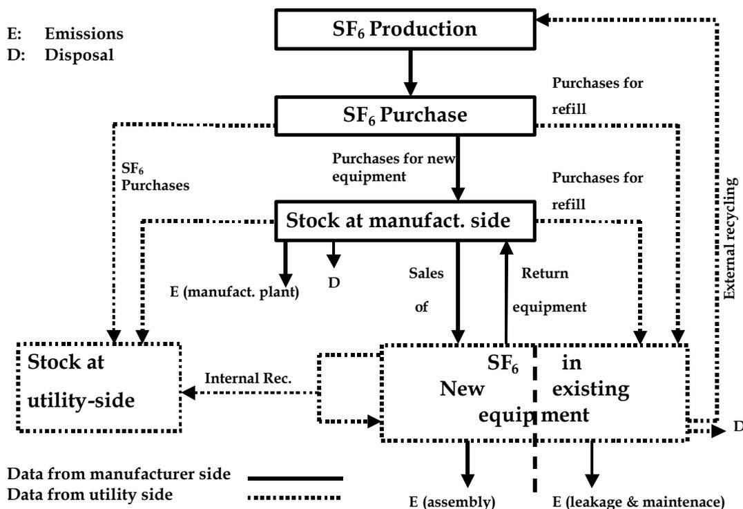
Figure 2: Monitoring of SF<sub>6</sub> emissions from electrical equipment in Germany
