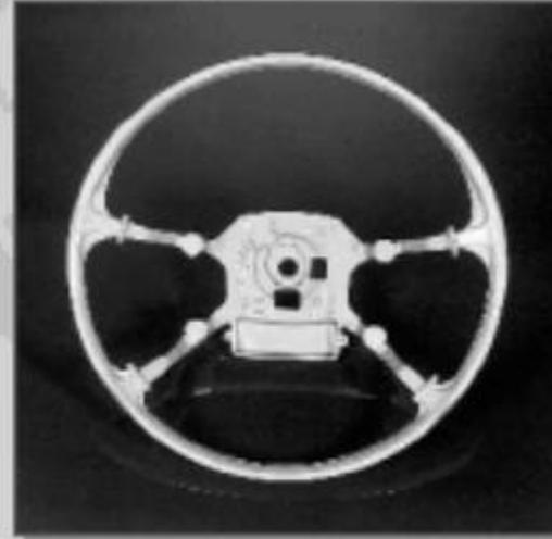
Steel Welded Armature
