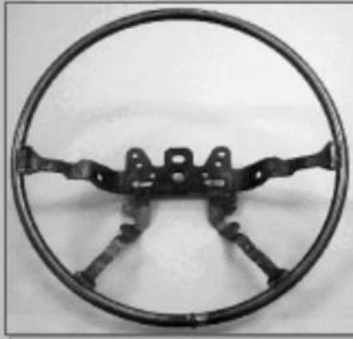
Full Die Cast Mg Armature
