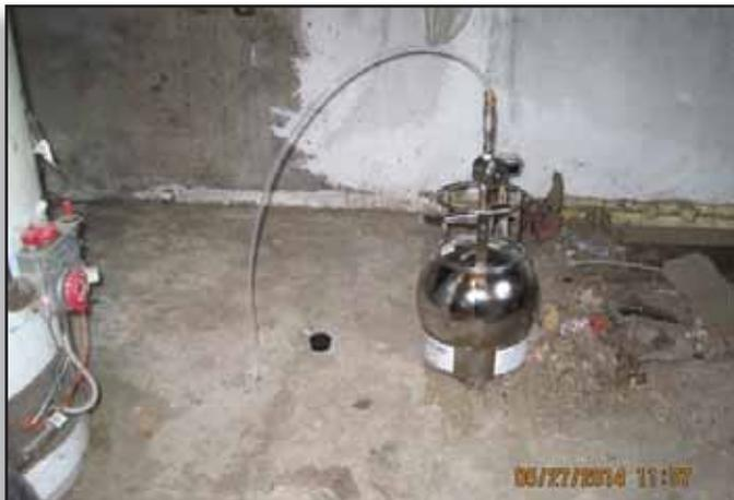
*SUMMA canister used to collect a sub-slab sample.*
