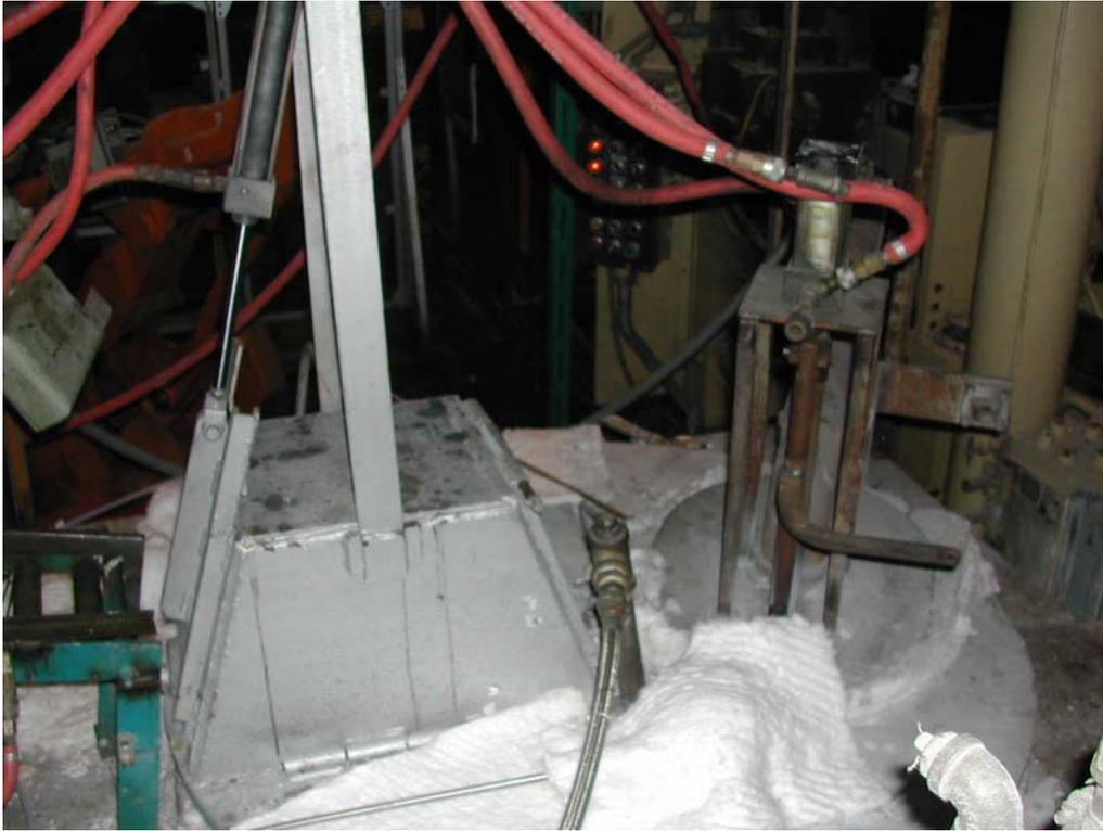
**Figure 1-1. Die Casting Machine Crucible at Lunt Manufacturing**
