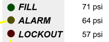
A quick flash on the next lower LED indicates a leak condition has been detected.
