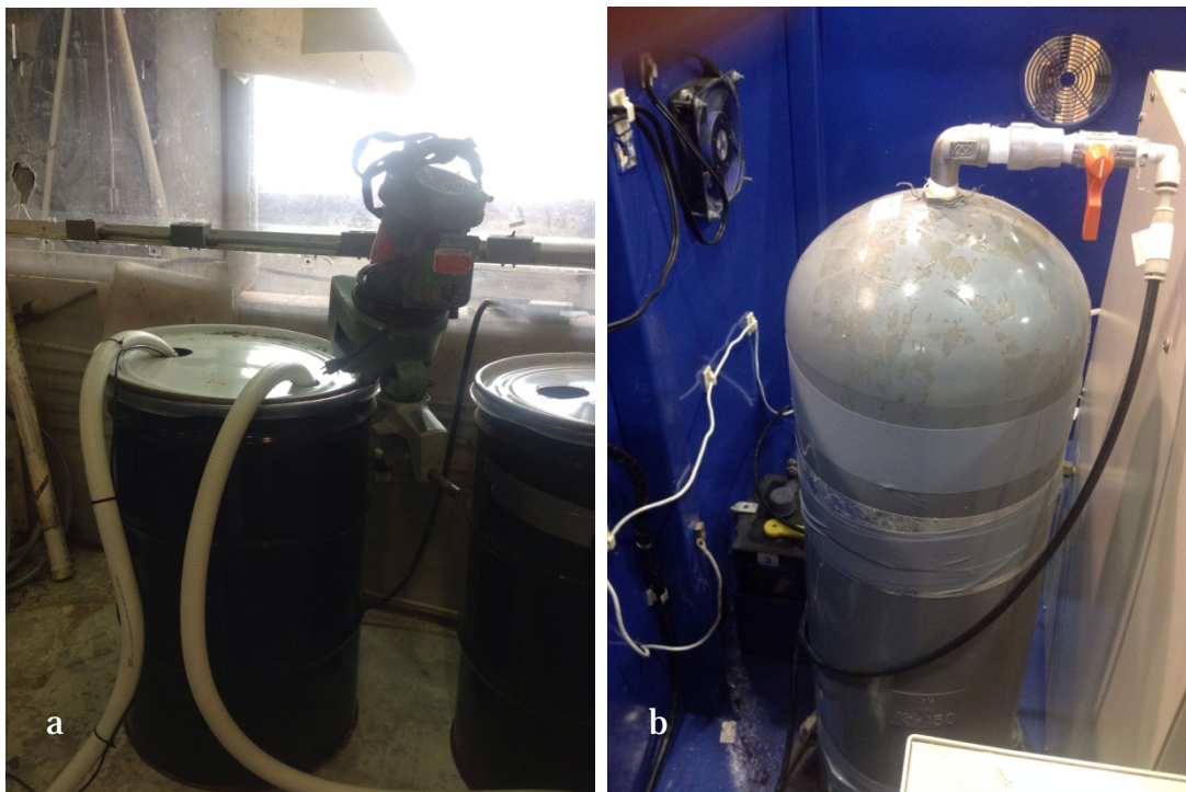
Figure 2. Propeller mixer (a) and on/off valve for superoxide reservoir (in "off" position, b).
