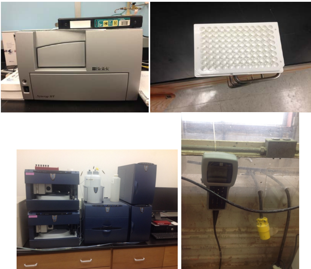
Figure 3. Some of the analytical instruments used in this project. Assay plate reader (upper left) and 96 well plate used for the superoxide dimutase assay (upper right), which were used to semi-quantitatively measure superoxide concentration, and dionex ion chromatograph used for nitrate and nitrite measurements (a similar system was set up for cation measurements and used for ammonium analysis) (lower left). Water quality meter for pH, conductivity, dissolved oxygen (DO), percent oxygen saturation (DO%), and oxygen-reduction potential (ORP) (lower right).
