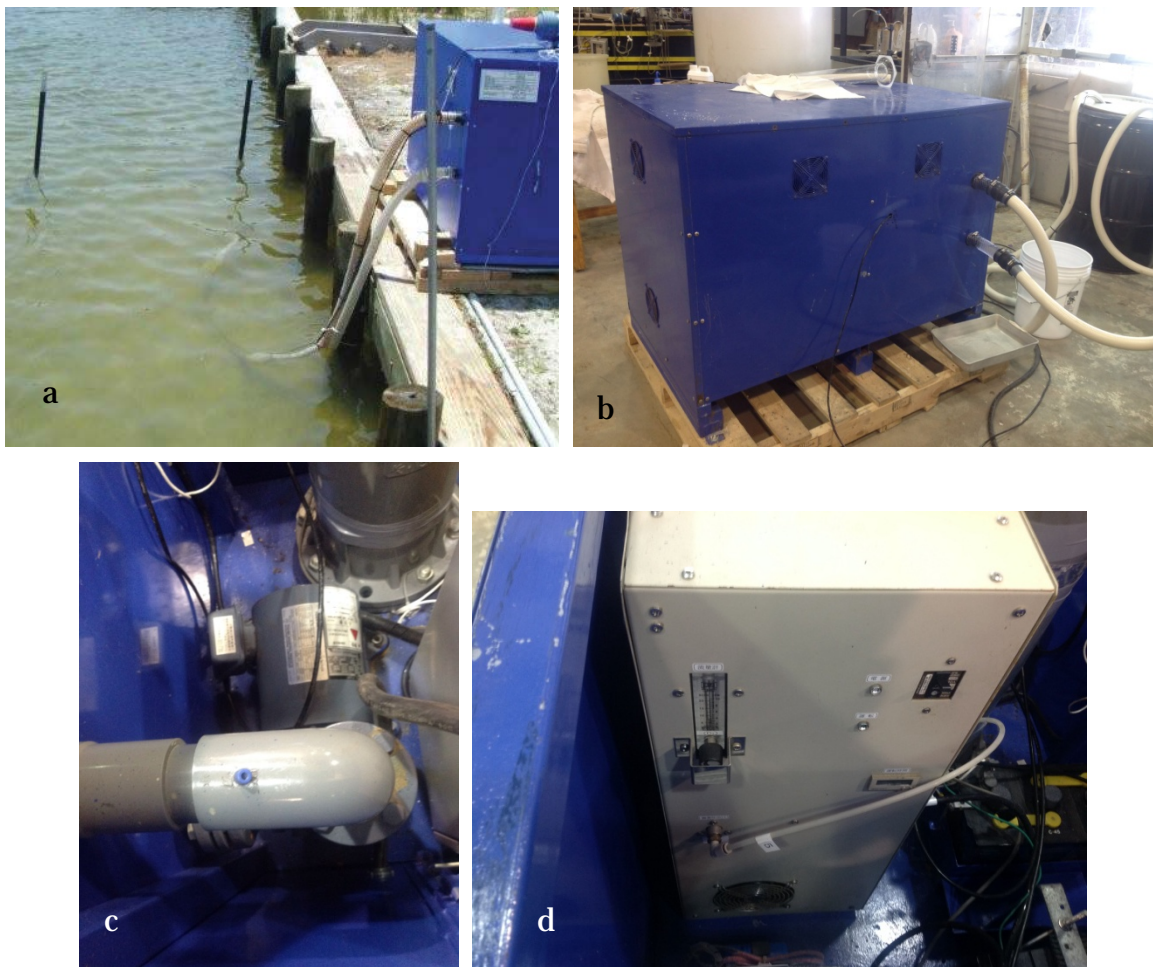
Figure 1. Field deployment of the KRIA water treatment system (a), and KRIA in laboratory (b), recirculation pump (c), and superoxide generation system (d).
