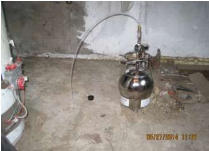
This device, called a SUMMA canister, collects sub-slab samples.
