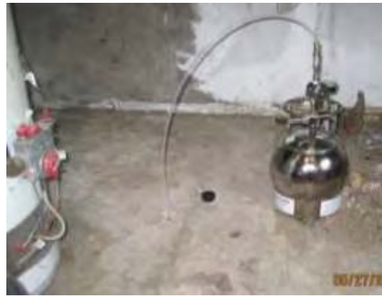
Photograph shows a SUMMA canister used to collect a sub-slab sample.
