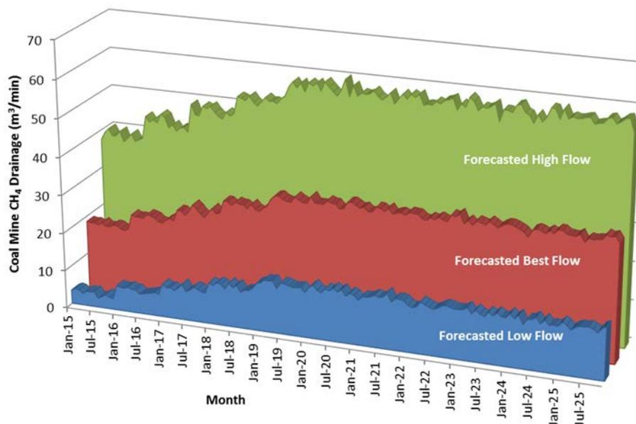
**Figure ES-1: Mahui Mine Forecasted Coal Mine Methane Drainage Available for Use (m<sup>3</sup>/min)**
