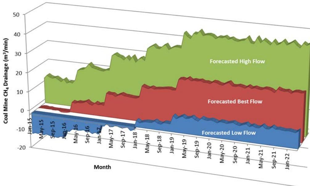
**Figure ES-2: Pingshang Mine Forecasted Coal Mine Methane Drainage Available for Use (m<sup>3</sup>/min)**
