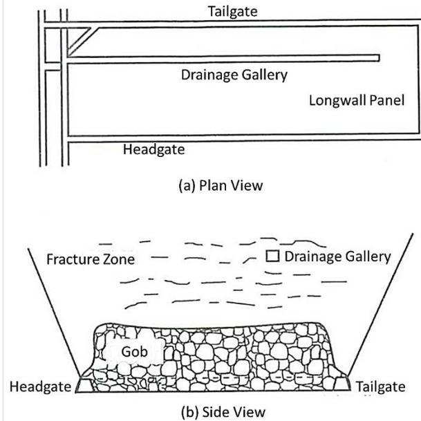
**Figure 3-3: Schematic Diagram of Existing Drainage System**
