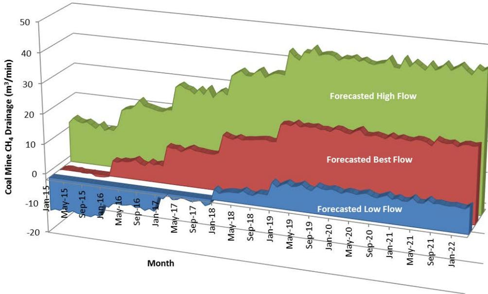
**Figure 4-7: Pingshang Mine Forecasted Coal Mine Methane Drainage Available for Use (m<sup>3</sup>/min)**
