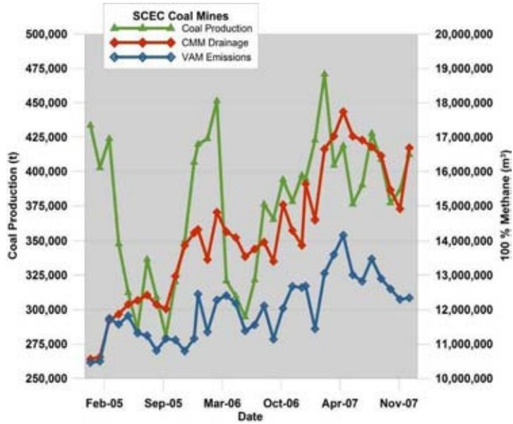
**FIGURE 5: SUMMARY OF SEEC COAL MINES COAL PRODUCTION AND VOLUME OF METHANE LIBERATED THROUGH DRAINAGE AND VENTILATION AIR**
