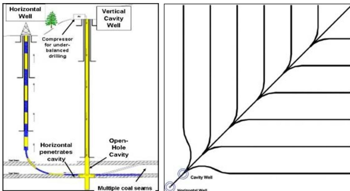
**Figure 4-21: Horizontal Pinnate Well Schematic**
