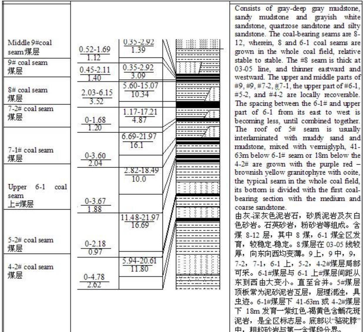
Figure 1-7: Detailed Coal Stratigraphy at Liuzhuang mine
