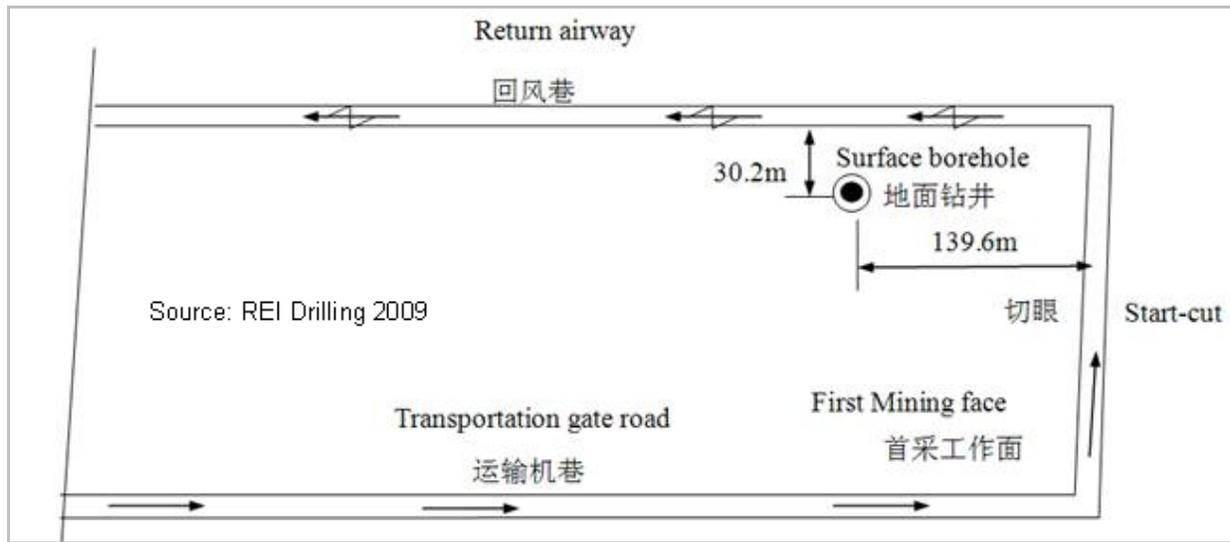
Figure 4-23: Surface to Horizontal Gob Borehole Drilled at Liuzhuang mine
