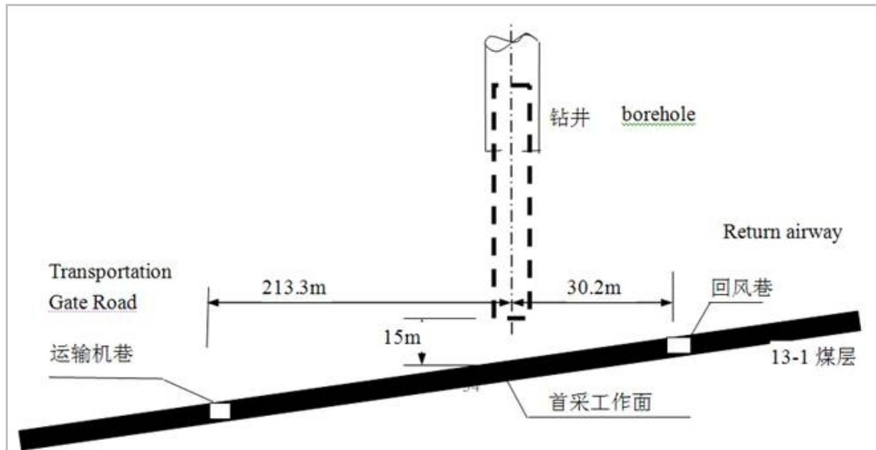
Figure 4-24: Surface to Horizontal Gob Borehole
