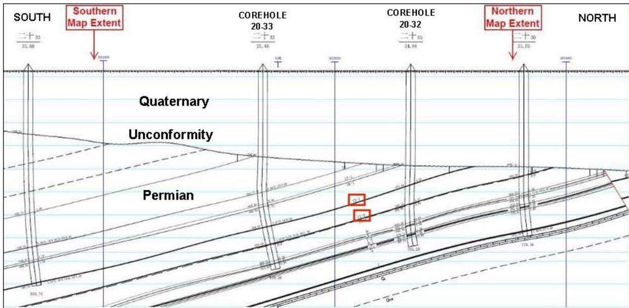
Figure 2-15: Expanded Section of N-S Cross-Section across Liuzhuang mine
