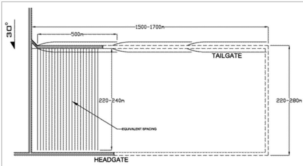
Figure 4-15: Alternative Drainage Drilling Scenario No.1
