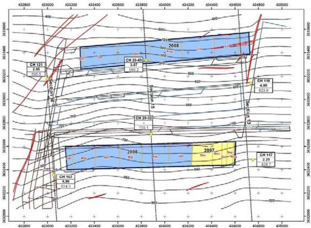
Figure 2-13: Structure and Depth to Seam 2-11 at Liuzhuang Mine
