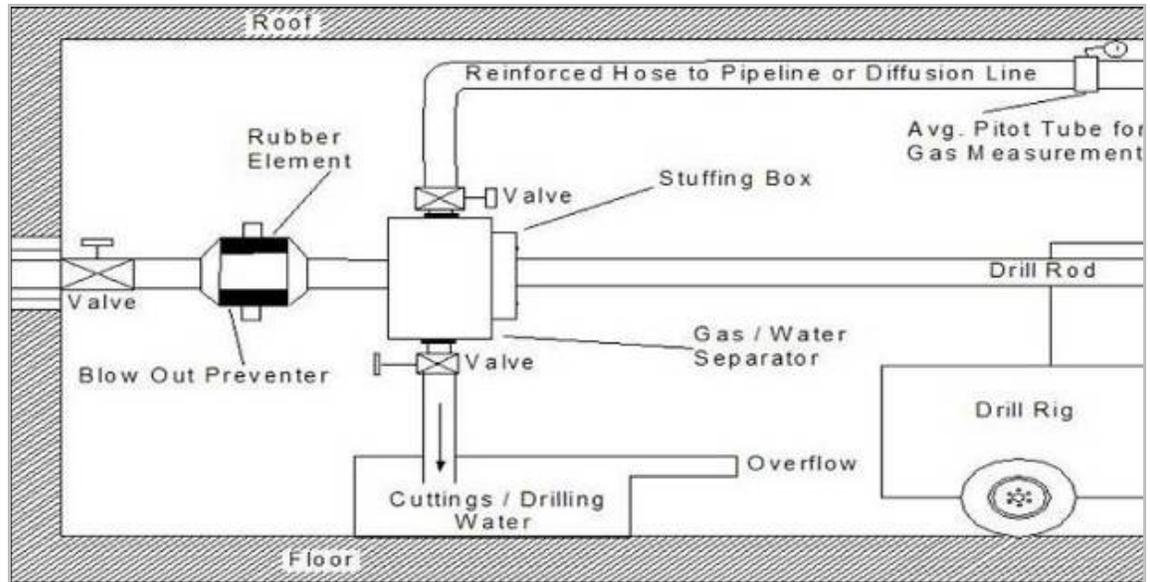
**Figure 6-3: Proposed Borehole Drilling Equipment and Procedures**
