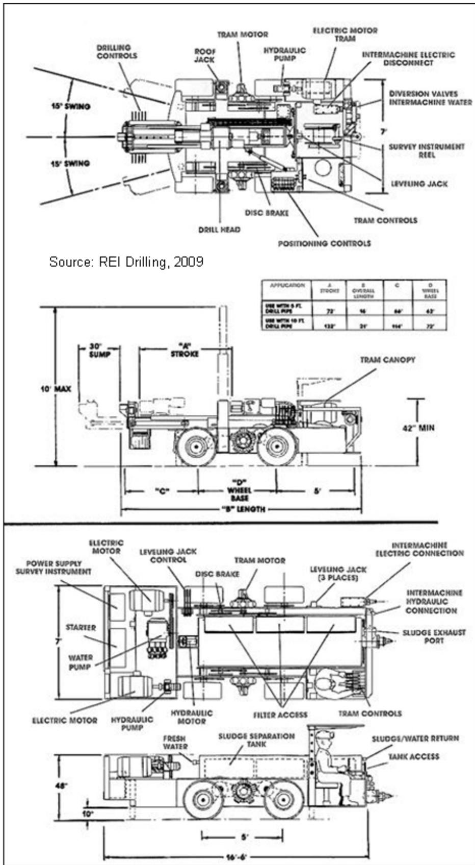
Figure 6-5: Schematic of Drilling Setup for Drilling Long (1000 m) Boreholes
