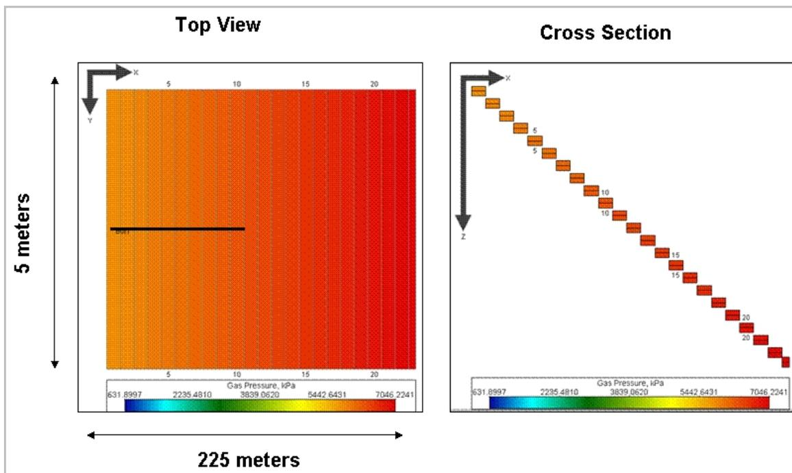
Figure 4-10: Reservoir Simulation Model of the Current Liuzhuang mine degasification borehole
