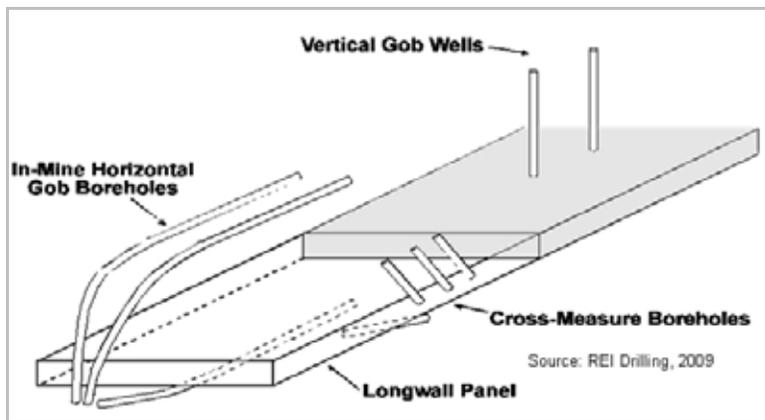
**Figure 6-1: Preliminary Engineering Strategy for Borehole Drilling at Liuzhuang mine**
