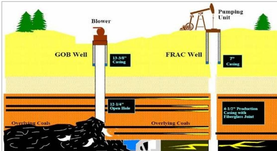
Figure 4-20: Vertical Frac Well Schematic
