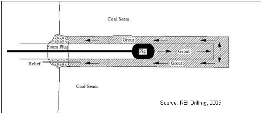
Figure 6-9: Grout Injection Process for Borehole Casing Completion
