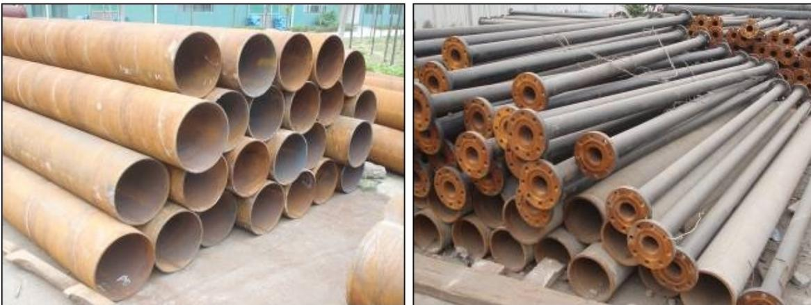
**Figure 4-5: Steel Pipe Used in the Underground-to-Surface CMM Pipeline System**
