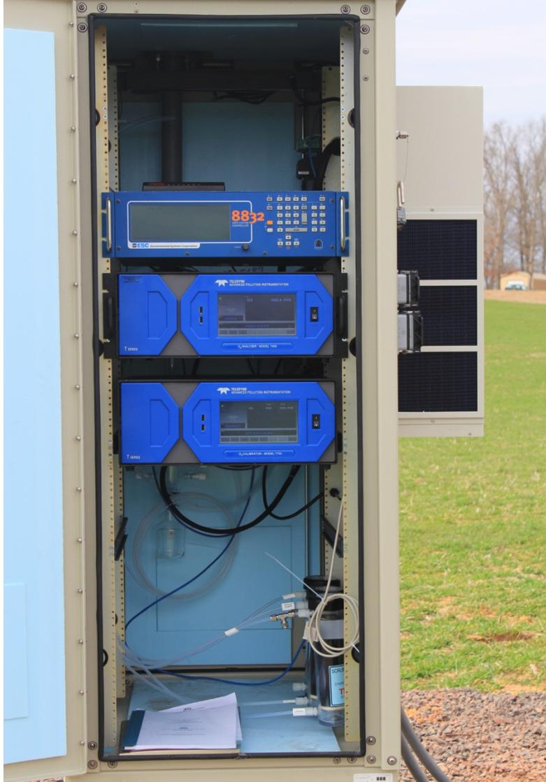
**Figure 4-2 – Typical SO<sub>2</sub> Monitoring Station Set-up**
