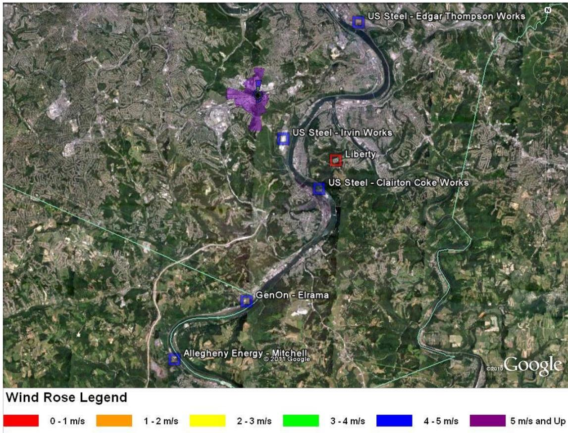
The wind is primarily out of the west and south. There is also a secondary maximum out of the north. This wind profile follows the synoptic wind flow over southwestern Pennsylvania. Stronger winds exist at this monitoring station because the wind is not undergoing any friction because it is not impacted by higher terrain.
