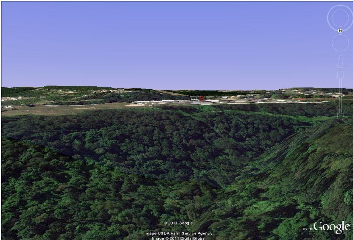
From Figure 29 (which looks north to south), one can see that the Liberty air monitoring station sits on top of a hill. However, there is higher terrain surrounding the monitor, creating valley like influences. The main SO<sub>2</sub> sources in the region are at lower elevation as they sit down within the river valley.
