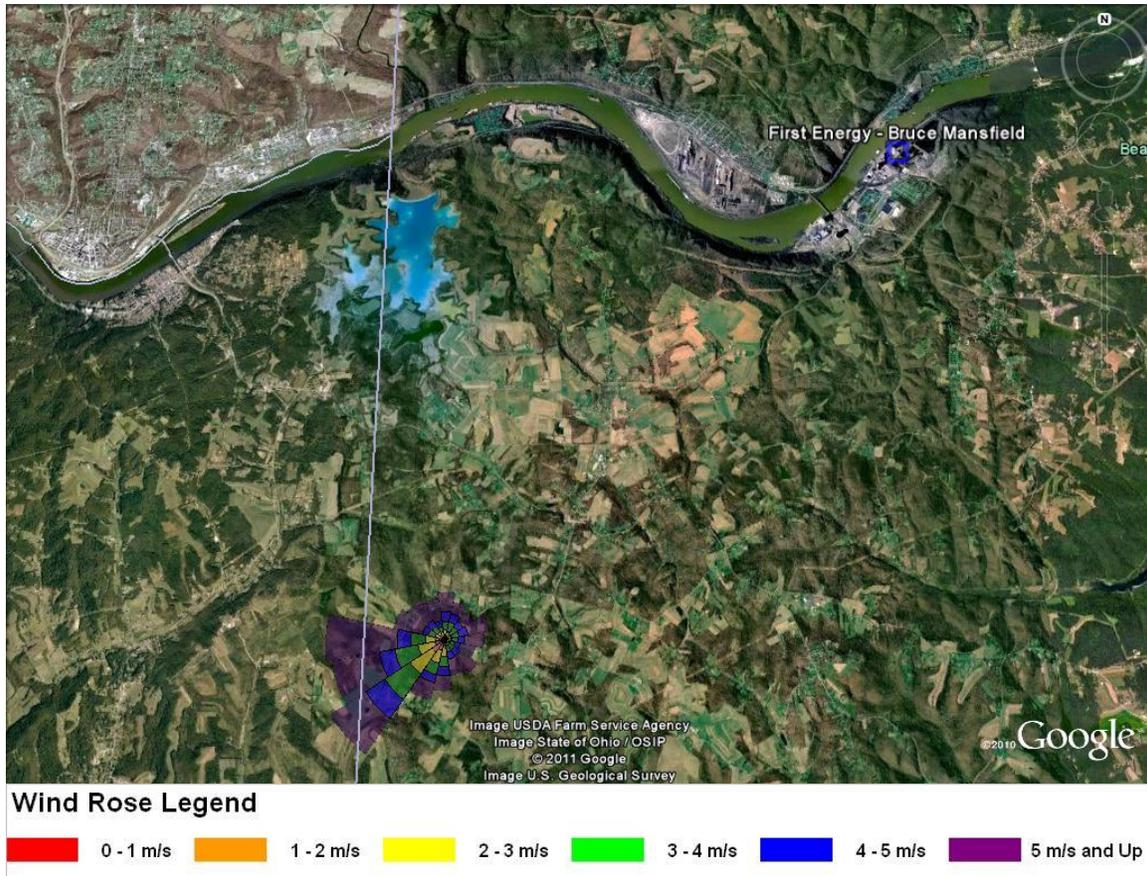
The wind is primarily out of the west and southwest. This wind profile follows the synoptic wind flow over the region and is not surprising by seeing Figure 18 above, which shows that there is not any significant terrain that is influencing the wind measurements.
