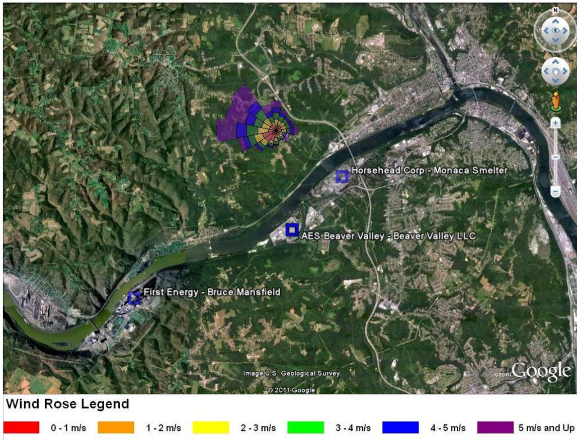
The wind is primarily out of the west and northwest. This wind profile follows the synoptic wind flow over the region and is not surprising by referencing Figure 12 above, which shows that there is not any significant terrain that is influencing the wind measurements.
