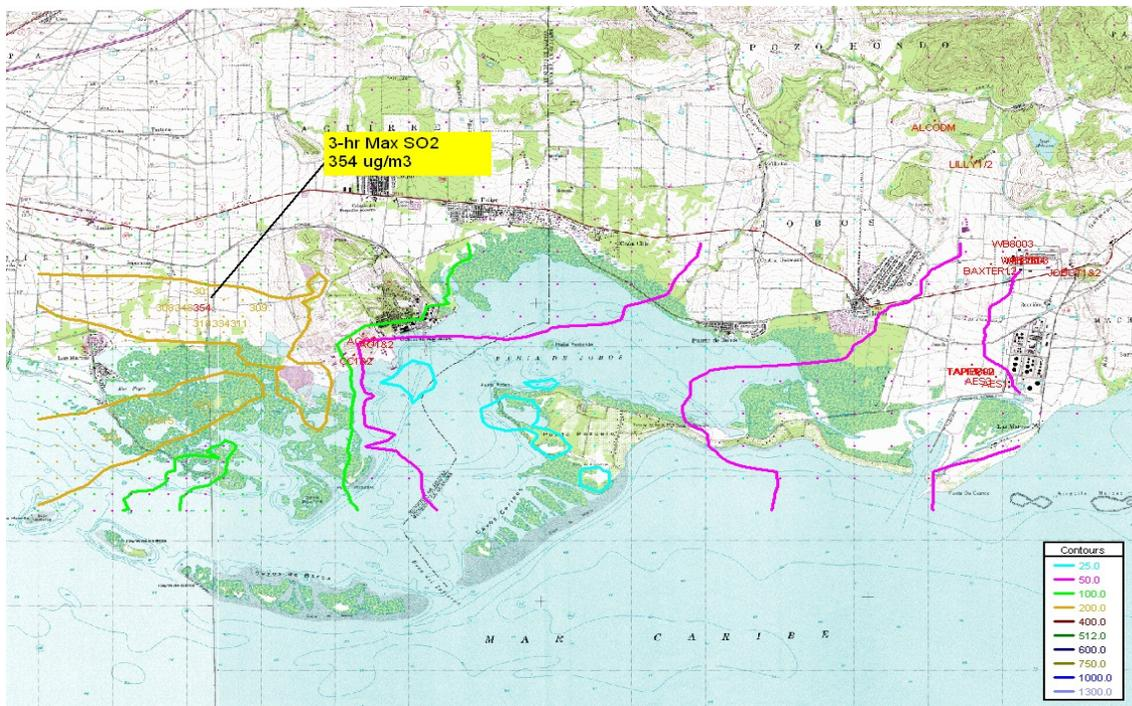
**Figure 4: AERMOD 3-hour SO<sub>2</sub> Modeling Results, PREPA Aguirre**
