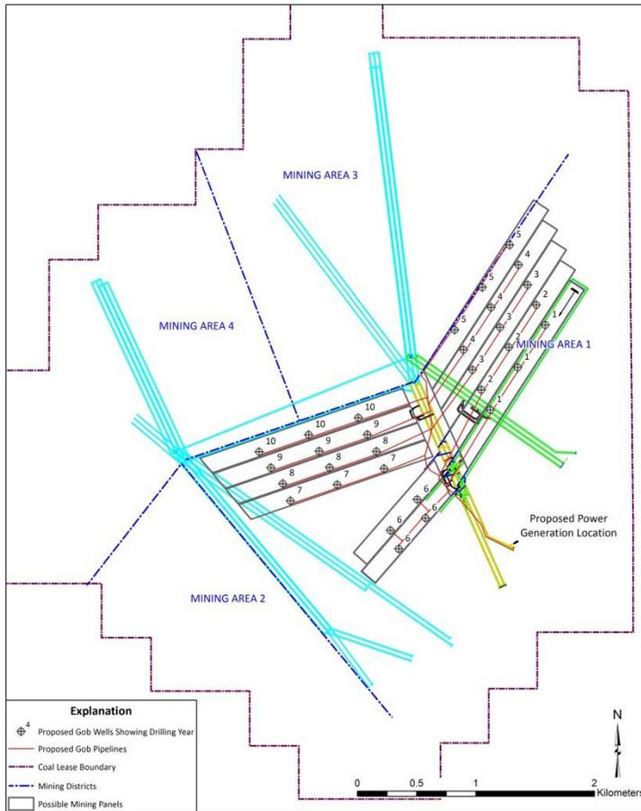
Figure 14: Layout of Proposed Gob Drainage Wells
