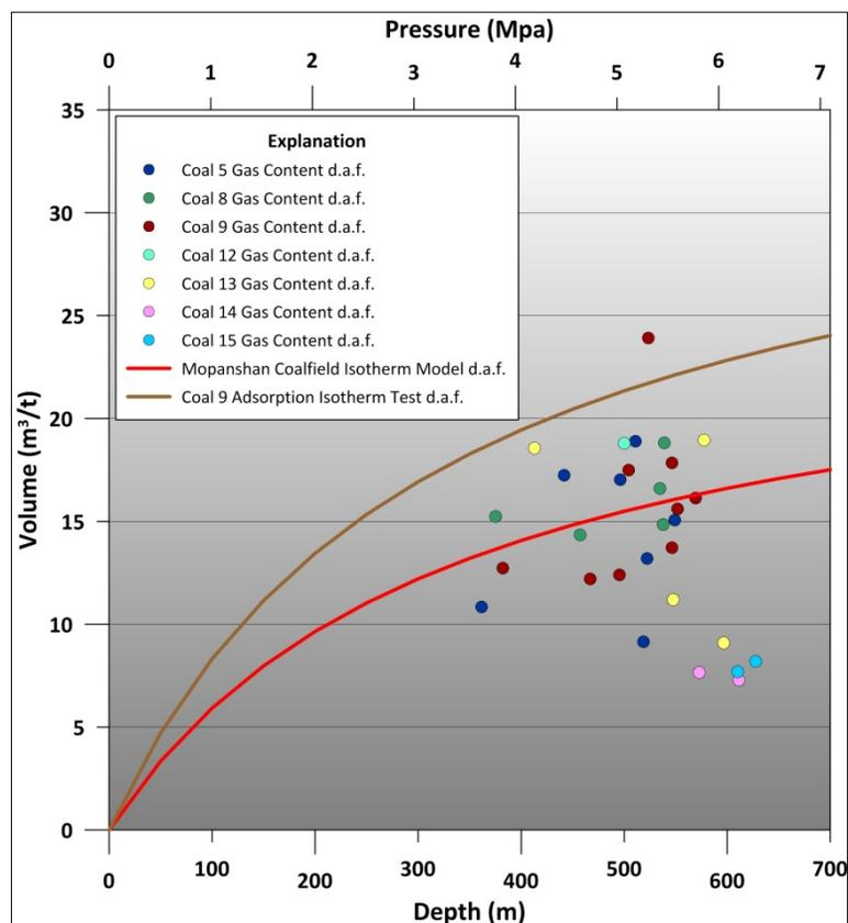
Figure 7: Adsorption Isotherm Curves and Gas Content Points
