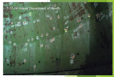
Destructive testing on at least one of the tanks to assess condition of outside of tank wall
