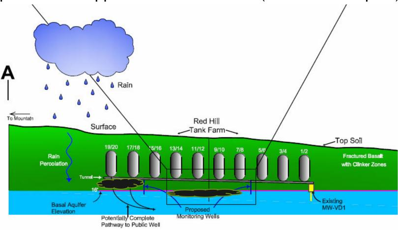
Step 3: Install additional monitoring wells as needed.
