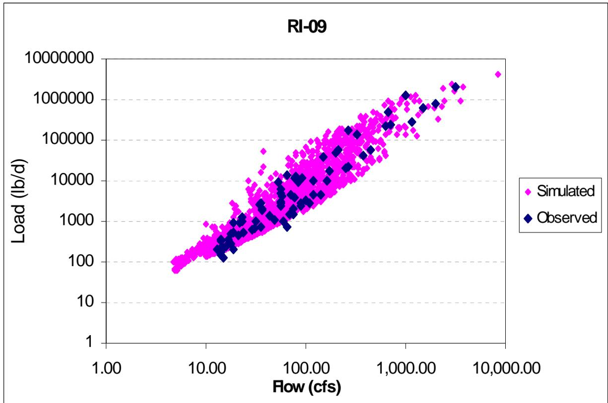
Figure 2. Simulated and observed sediment loading curves for the Menomonee River at sampling site RI-09 at Milwaukee for 1994-1998.
