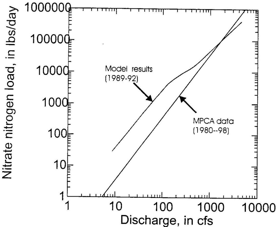
Figure 2. Simulated and observed nitrate loading curves for Cottonwood River near New Ulm, Minnesota.
