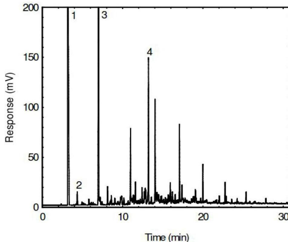
Figure 3.5.1 Chromatogram of 2.0 mg/mL kerosene in the extraction solvent. (key: (1) CS<sub>2</sub>, (2) benzene, (3) DMF, (4) p-cymene)
