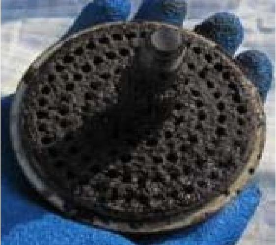
Retainer and valve with paraffin wax buildup
