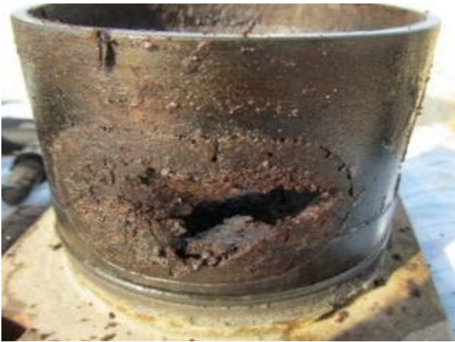
Retainer and valve with paraffin wax buildup
