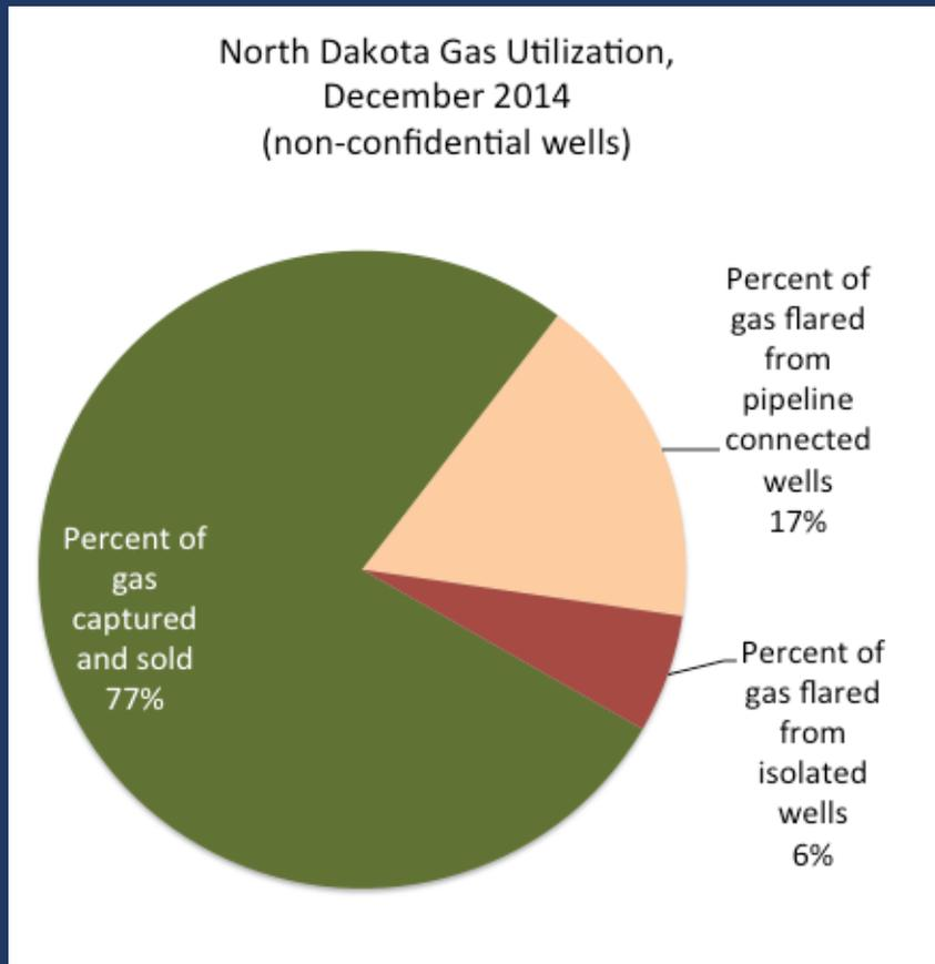
Both isolated well flaring and pipeline connected flaring are significant in tight oil basins in the U.S.
