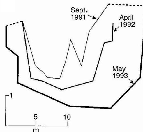
Figure 40. Surveyed stream channel cross-sections taken downstream of an urbanizing area on Borrego Canyon Wash, CA.
