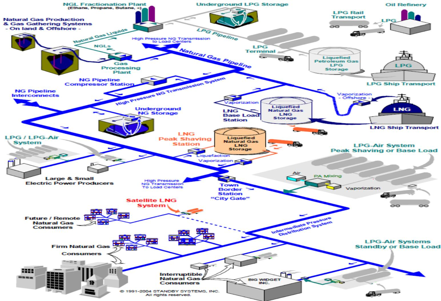
3 From wellhead to burner tip, this graphic shows the pieces and parts of a natural gas energy grid. The sections in orange show a typical LNG peak shaving plant location.
