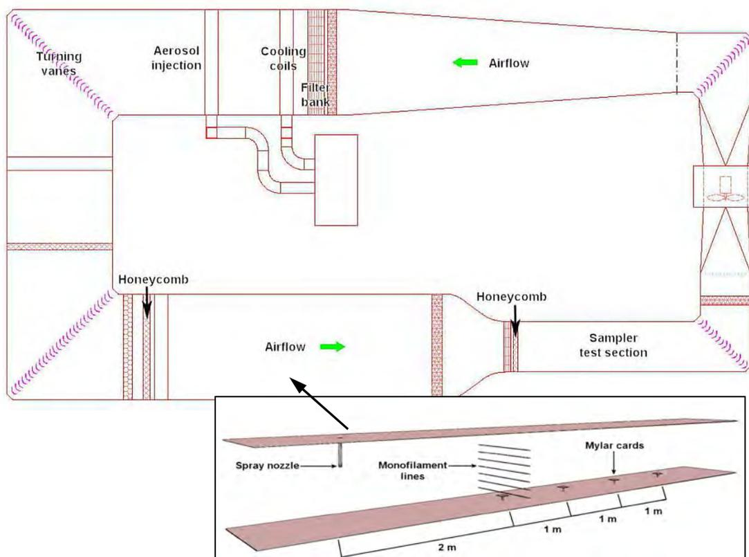
**Figure 2. EPA's aerosol wind tunnel (AWT).**
