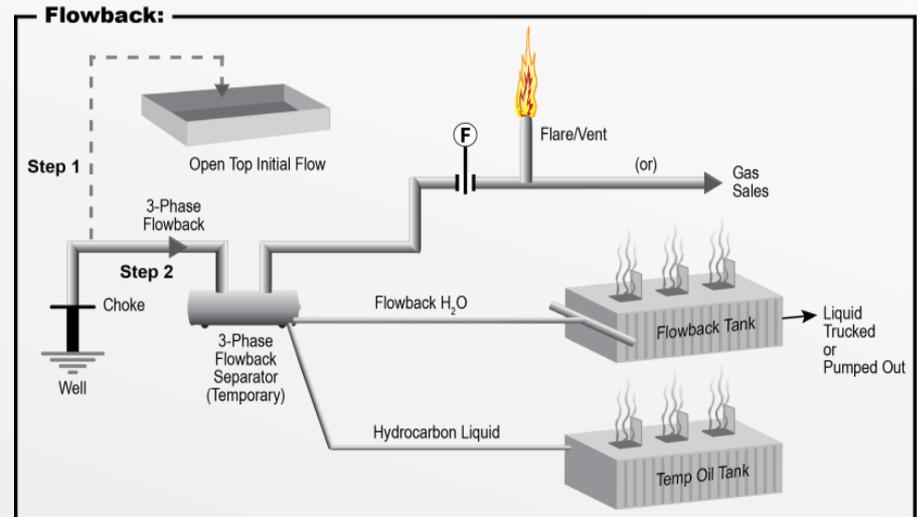
*Note: Sand Filter may be installed upstream of Separator. Also, there may be 2-stage (HP, LP) Separation.*
