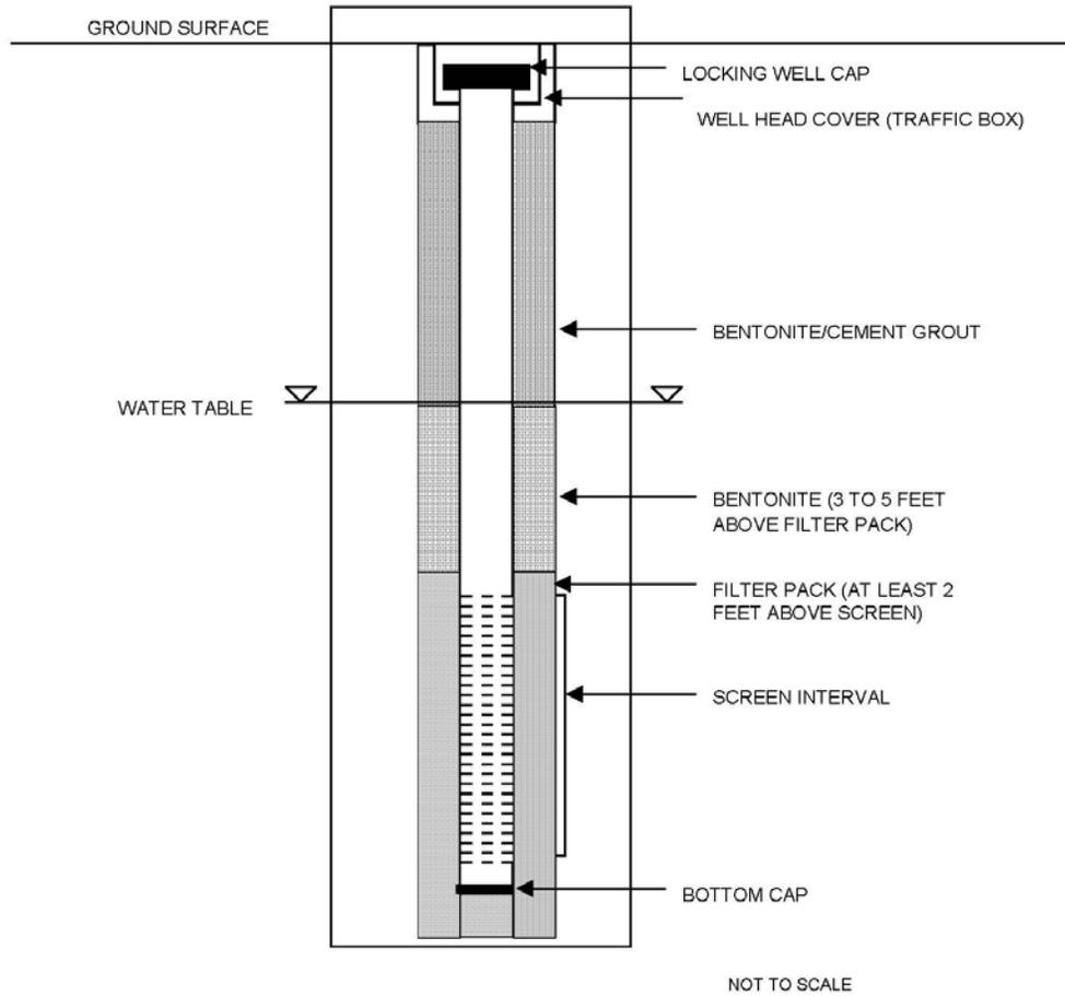
Figure I-C-1-2: General Cross Section of Monitoring Well, Confined Water Bearing Zone
