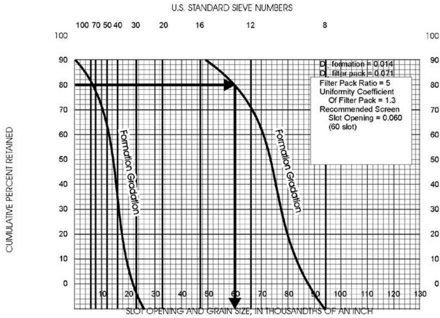
Figure I-C-1-3: Selecting Well Intake Slot Size Based on Filter Pack Grain Size
