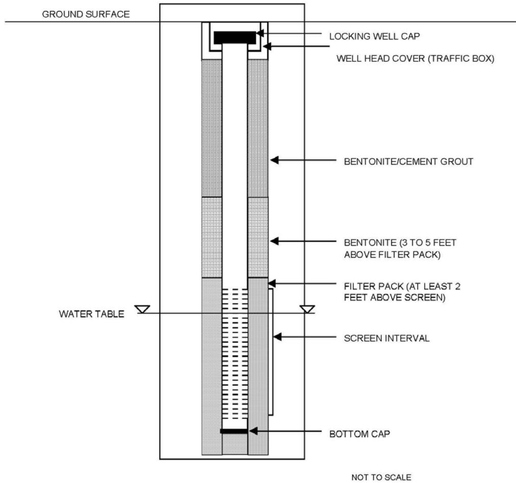
Figure I-C-1-1: General Cross Section of Monitoring Well, Unconfined Water Bearing Zone
