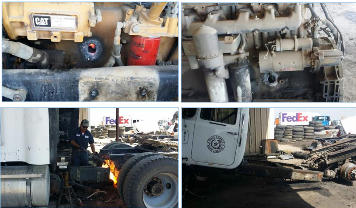
Figure 4-1. Holes bored into the engine blocks of the two replaced vehicles (upper panels) and severed frame rails in the two replaced vehicles (lower panels).
