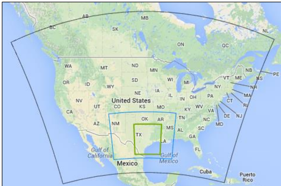
Figure 2-21. TCEQ 36/12/4 km CAMx nested modeling grids for the Texas ozone modeling of June 2012. 36 km grid is outlined in black. The 12 km grid outlined in blue, and the 4 km grid is outlined in green. TCEQ figure from http://www.tceq.texas.gov/airquality/airmod/rider8/modeling/domain .
