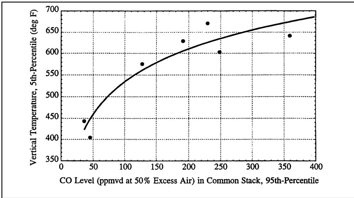
Figure A.16-3. CO Level (95<sup>th</sup> Percentile) in the Common Stack vs. Vertical Temperature Measurement (5<sup>th</sup> Percentile).
