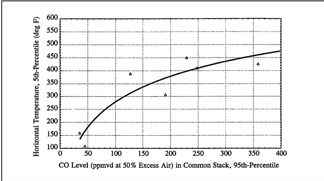
Figure A.16-2. CO Level (95<sup>th</sup> Percentile) in the Common Stack vs. Horizontal Temperature Measurement (5<sup>th</sup> Percentile).
