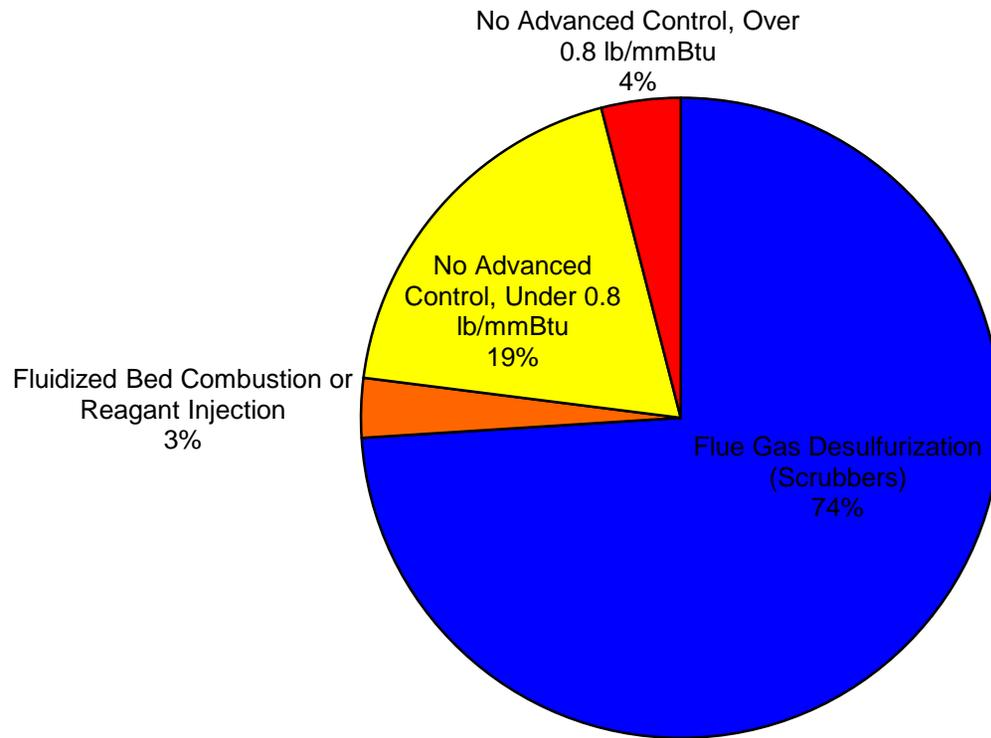
**Sulfur Dioxide Controls for 2015 ARP/CSAPR
