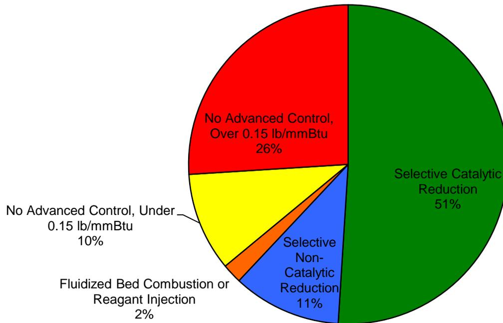
**Nitrogen Oxide Controls for 2015 ARP/CSAPR
