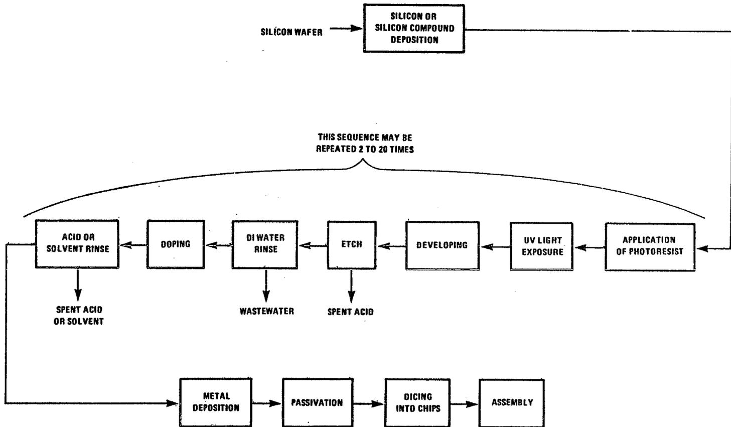
FIGURE 4-1. SILICON INTEGRATED CIRCUIT PRODUCTION
