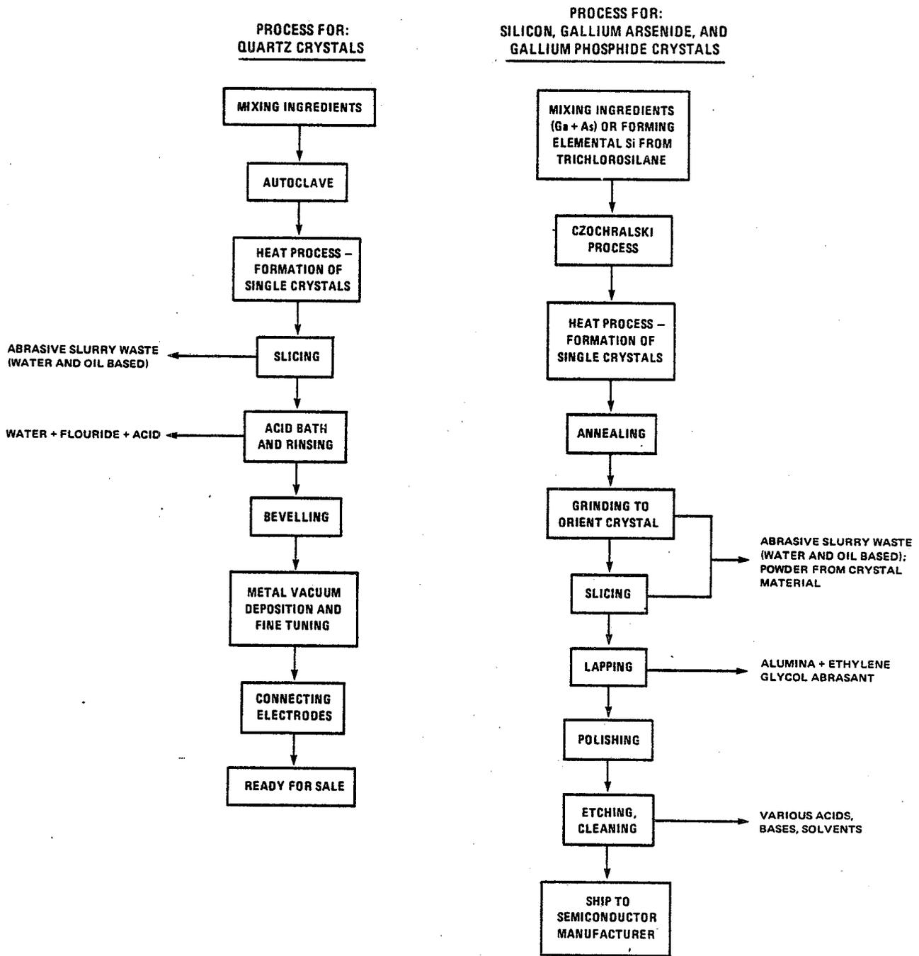
FIGURE 4-2. BASIC MANUFACTURING PROCESSES FOR ELECTRONIC CRYSTALS
