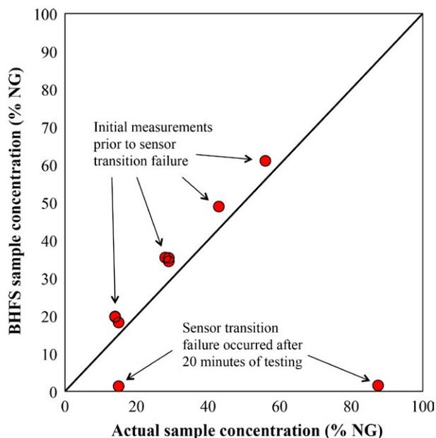
**Figure 5.** Performance of the BHFS used during the [1] study with NG composed of 90.8% CH<sub>4</sub>; instrument firmware had been upgraded to version 3.04 after that study but before this testing; calibration was 2 weeks old. Sensor transition failure set in after ~20 min of testing; this failure was eliminated once the BHFS was put through a calibration sequence (as opposed to just a response test). BHFS, Bacharach Hi-Flow Sampler; NG, natural gas.
