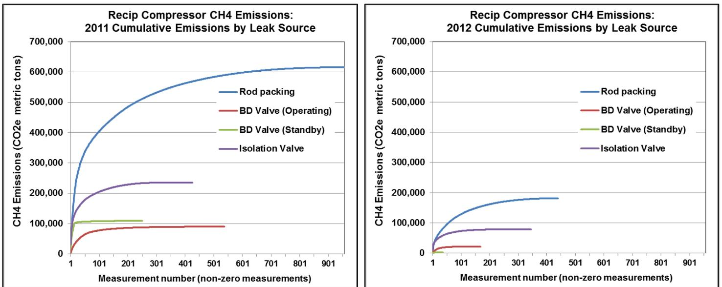
**Figure 6. Reciprocating compress emissions by source – mode combination: Rod packing (operating mode), blowdown valve (operating mode or standby-pressurized mode) and isolation valve (shutdown-depressurized mode).**
