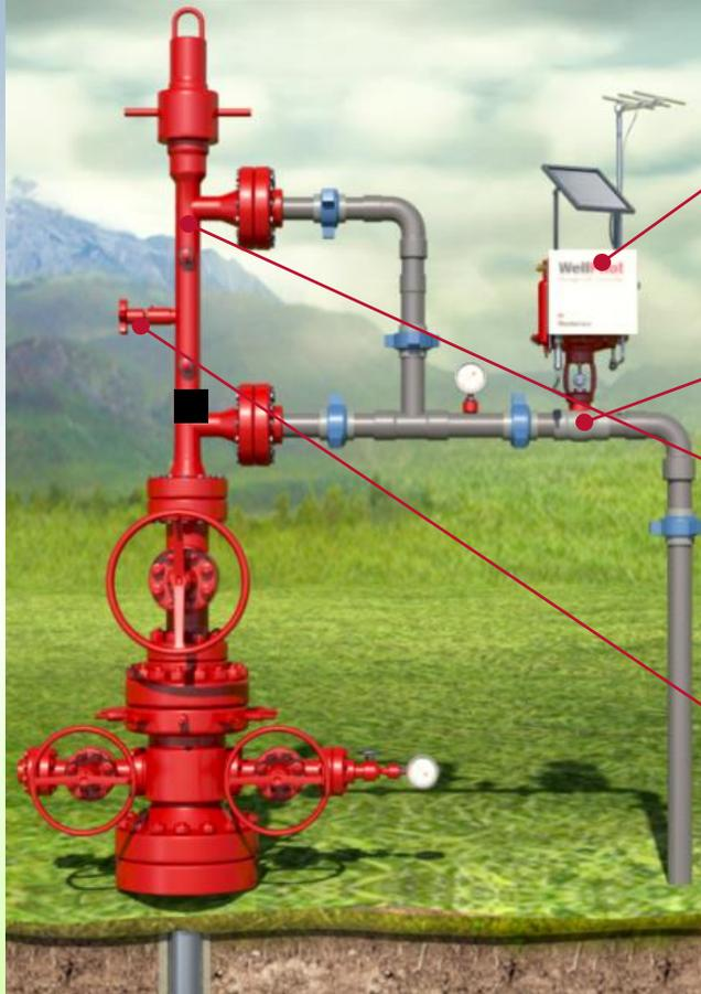
**Controller:** Electronic-based system with control parameters for opening and closing motor valves
