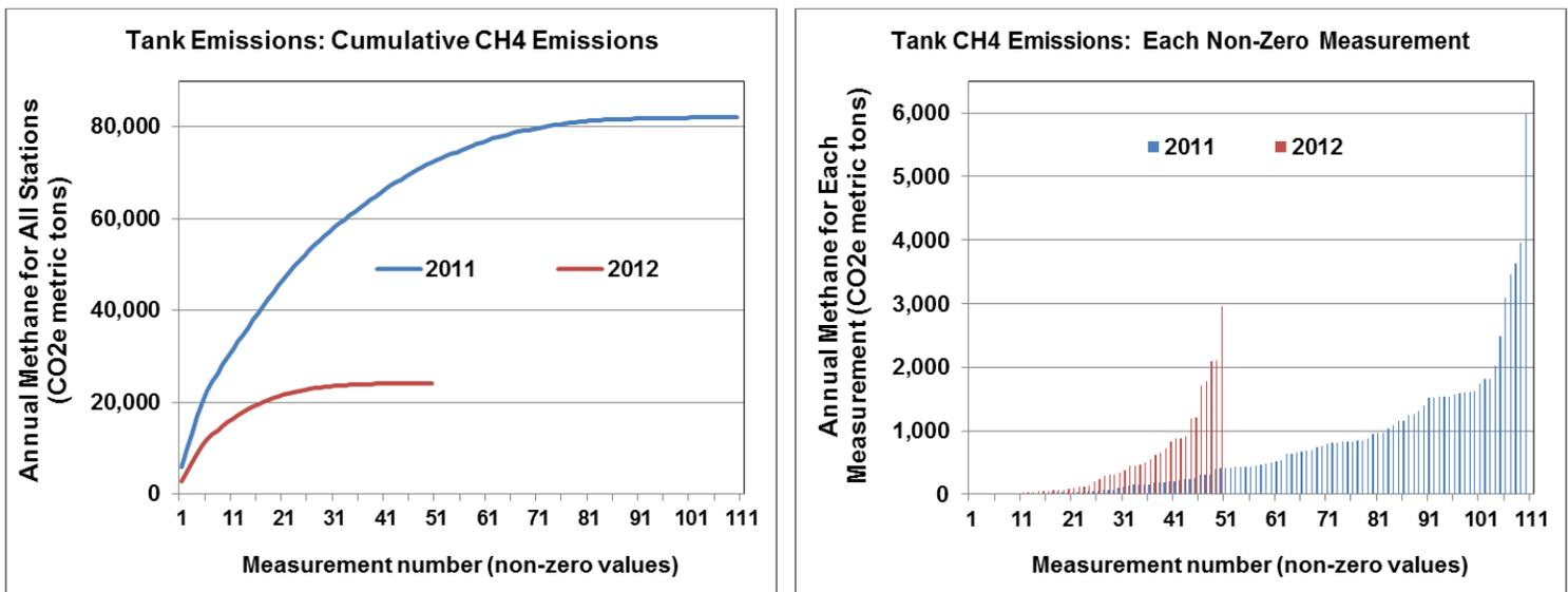
**Figure 6. Storage tank emissions from leaking dump valves in 2011 and 2012. Cumulative distribution of all non-zero measurements (left graph) and leak rate for each non-zero measurement (right graph).**
