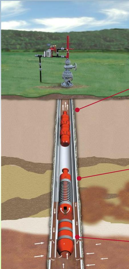
**Plunger:** Pig-type device that provides seal inside tubing to deliver fluid to surface
