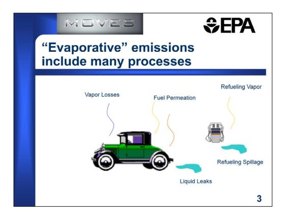
There are five basic non-exhaust processes which are included in the estimate for what is commonly called "evaporative" emissions. All of these sources involve fuel (hydrocarbons) that escape from the system and vaporize (evaporate) into the atmosphere. MOVES addresses each of these sources and makes an estimate of their impact on vehicle emissions.
