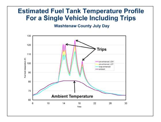
This figure illustrates how fuel tank temperature lags the ambient temperature during cold soak, rises when the vehicle is driven, peaks at the end of each trip, and declines during the Hot Soak period. The estimate of tank temperature is affected by vehicle type and technology.
