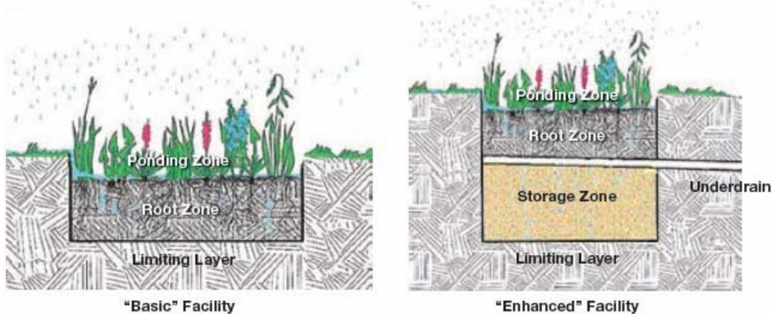
Figure 7. Basic bioretention models (Atchison et al. 2006)
