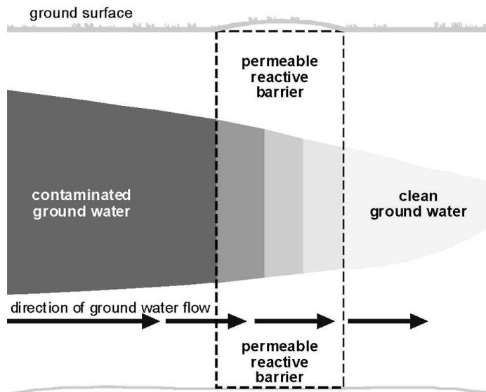
Figure 4. Permeable reactive barrier (EPA 1999)
