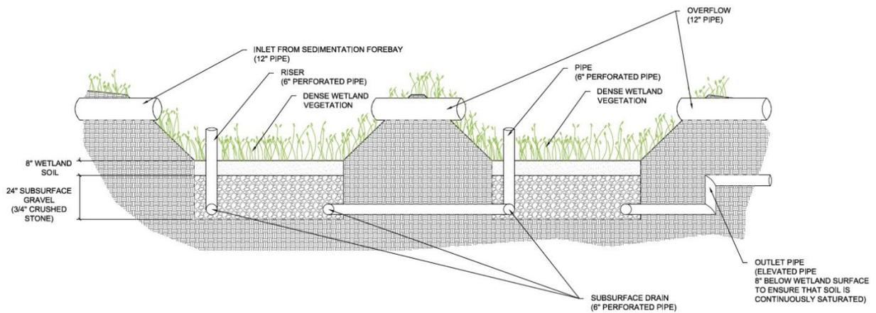
Figure 17. Gravel wetland schematic (CRWA 2009)
