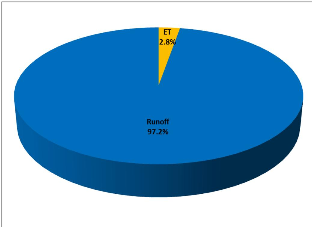
Figure 31. Overall water balance in the bioretention outflow at the Drive-In site
