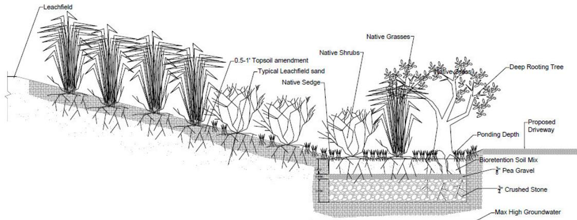
Figure 28. Cross-sectional view of the enhanced bioretention and phytotechnology area to be implemented at the Drive-In site (Cape Cod Commission/Tetra Tech)
