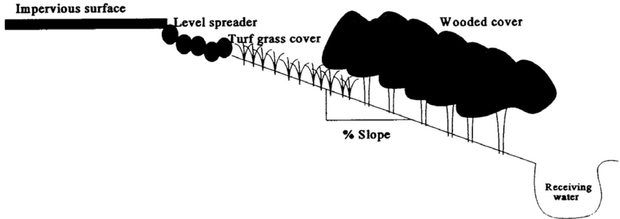
Figure 6. Diagram of a typical biofiltration strip (Clar et al. 2004)
