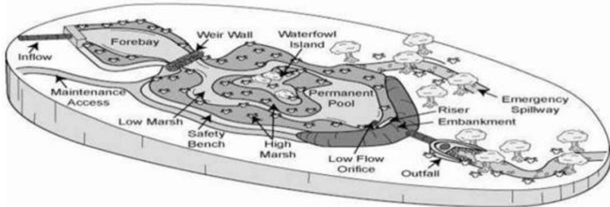
Figure 3. Typical plan view of a constructed wetland system (VADCR 2011)
