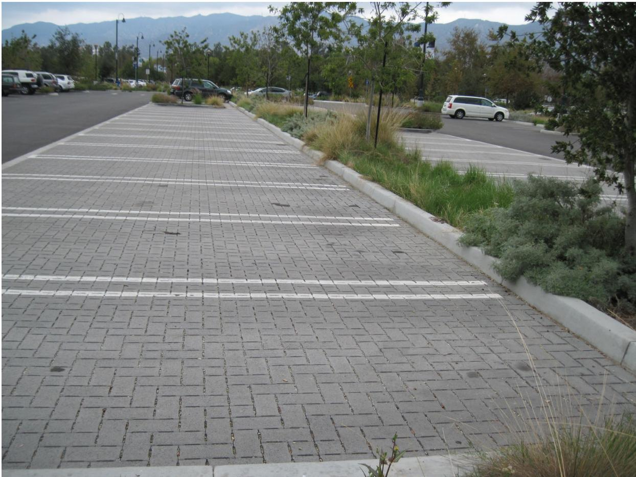
Figure 13. Permeable pavement in parking lot (Tetra Tech)
