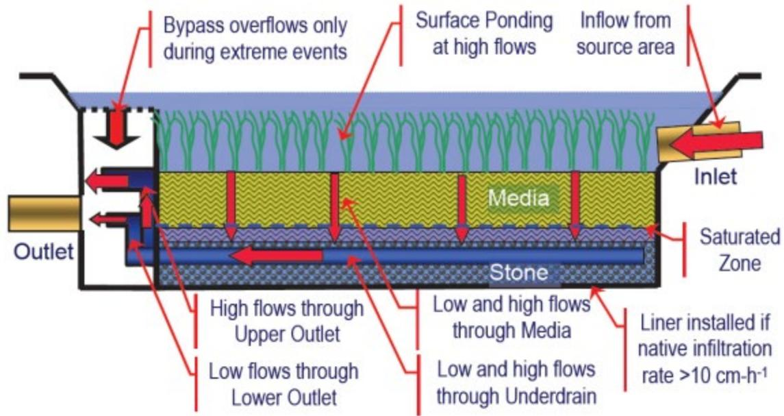
Figure 9. Advanced Bioretention adapted from Lucas & Greenway (2011a)
