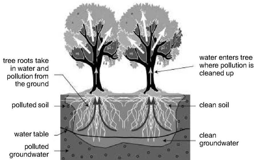
Figure 5. Typical phytoremediation process (EPA 2012)
