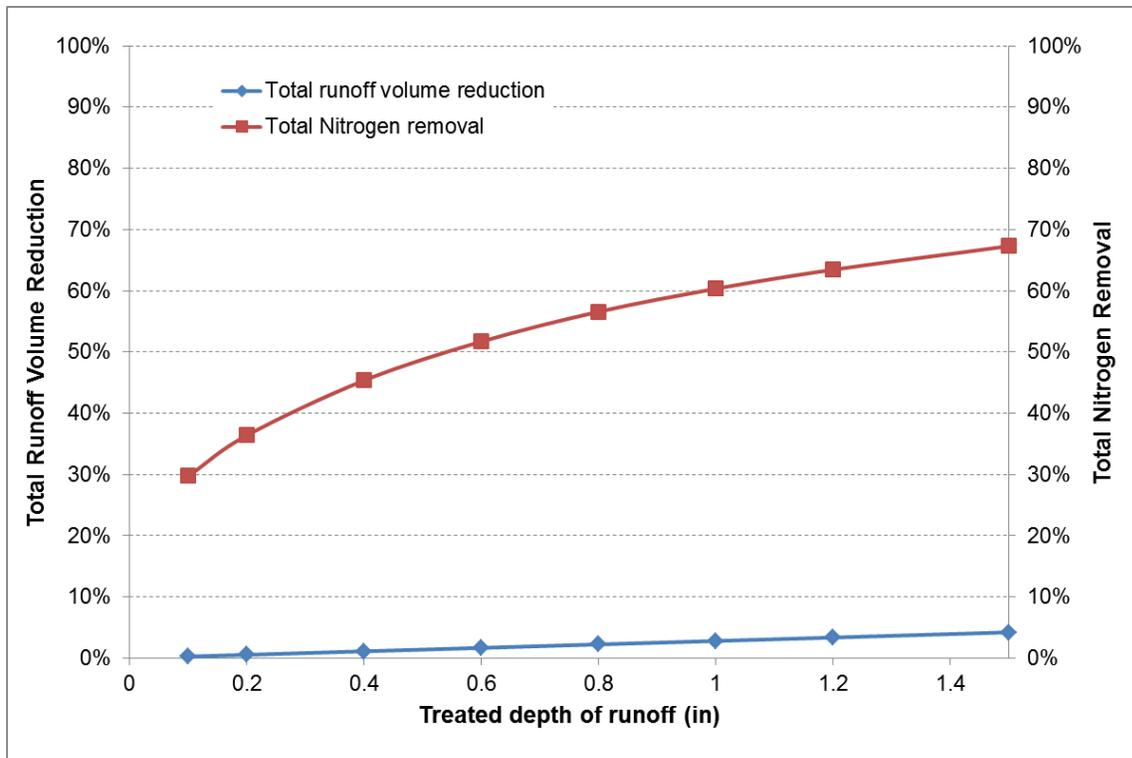
Figure 32. Simplified cost-effective analysis for sizing the enhanced bioretention at the Drive-In site
