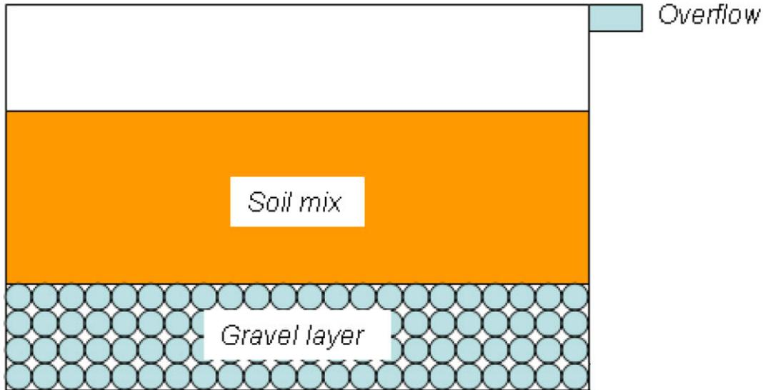
Figure 30. Schematic for representing the conventional bioretention into SUSTAIN (not to scale)
