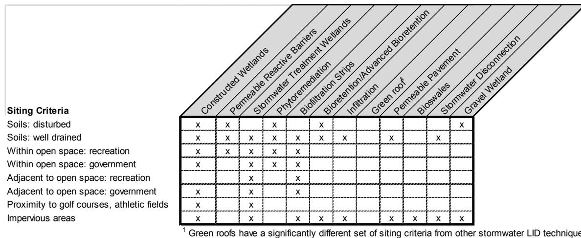
Figure 19. Revised Screening Process Matrix
