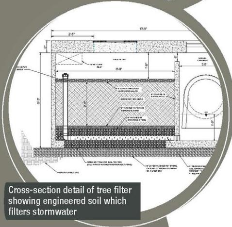
Cross-section detail of tree filter showing engineered soil which filters stormwater
