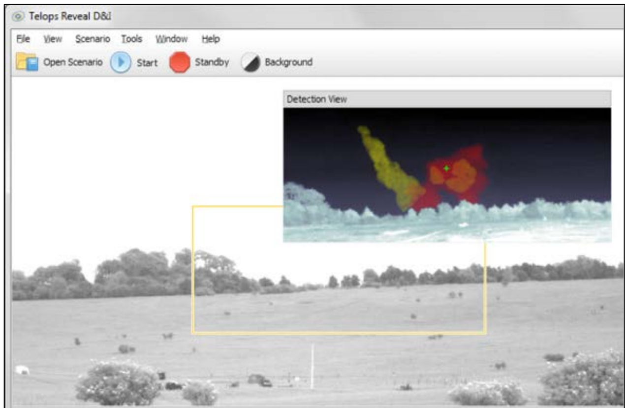
Figure 3.38. Example Telops Software Output Where the Detection View is the Total Radiance with the Gas Cloud Highlighted in False Color.
