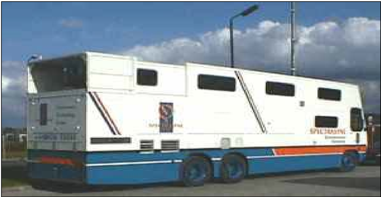
Figure 2-21. Mobile DIAL Unit
