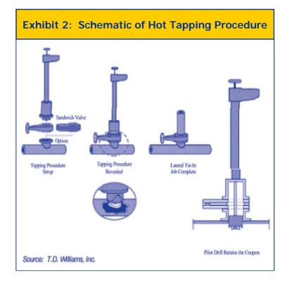
are also available that allow a hot tap to be performed by a single operator, without additional blocking or bracing.
