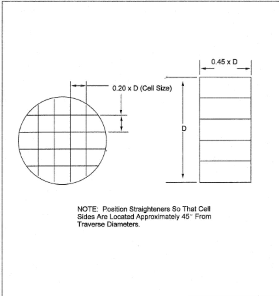
Figure 5D-1. Example of Flow Straightening Vanes.
