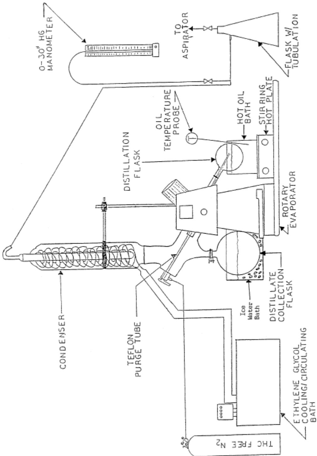
Figure 204F-1. VOC distillation system apparatus.
