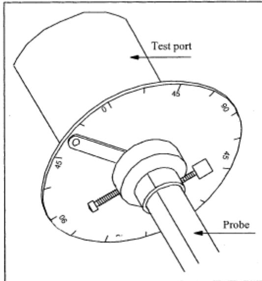
Figure 2G-5. Yaw angle protractor wheel and pointer.
