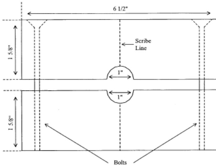
Figure 2G-4. Rotational position collar block.
