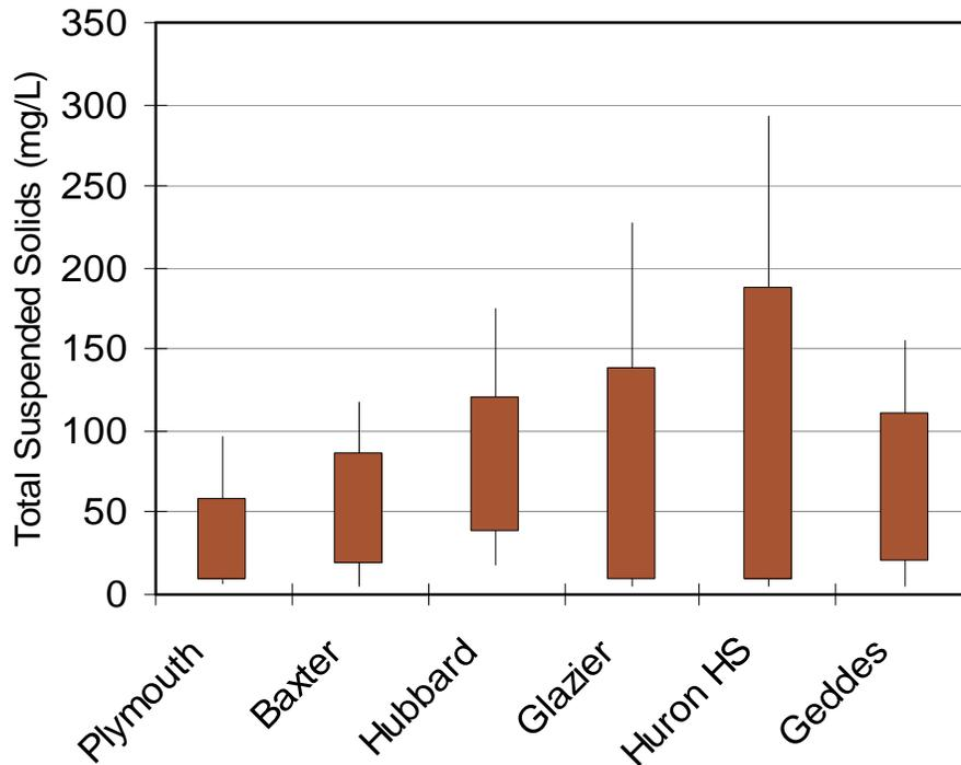
**Figure 5.6 Measured Dry and Wet Weather Total Suspended Solids Concentrations**
