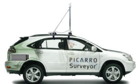
Picarro's leak detection technology is installed on cars, which allows surveyors to drive through neighborhoods to check for natural gas leaks.
