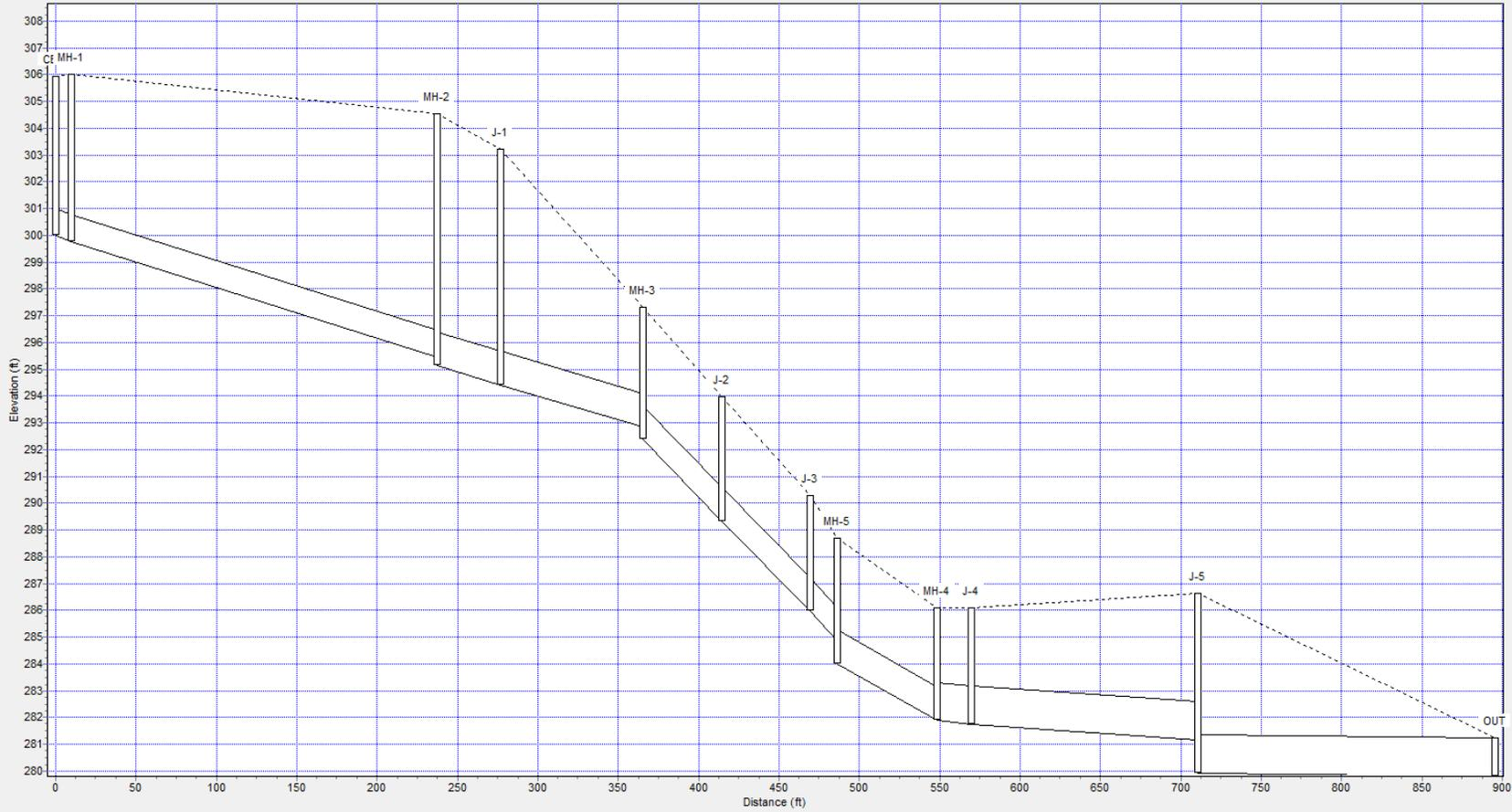
Figure 6. Hydraulic Profile of Main Trunk-Line
