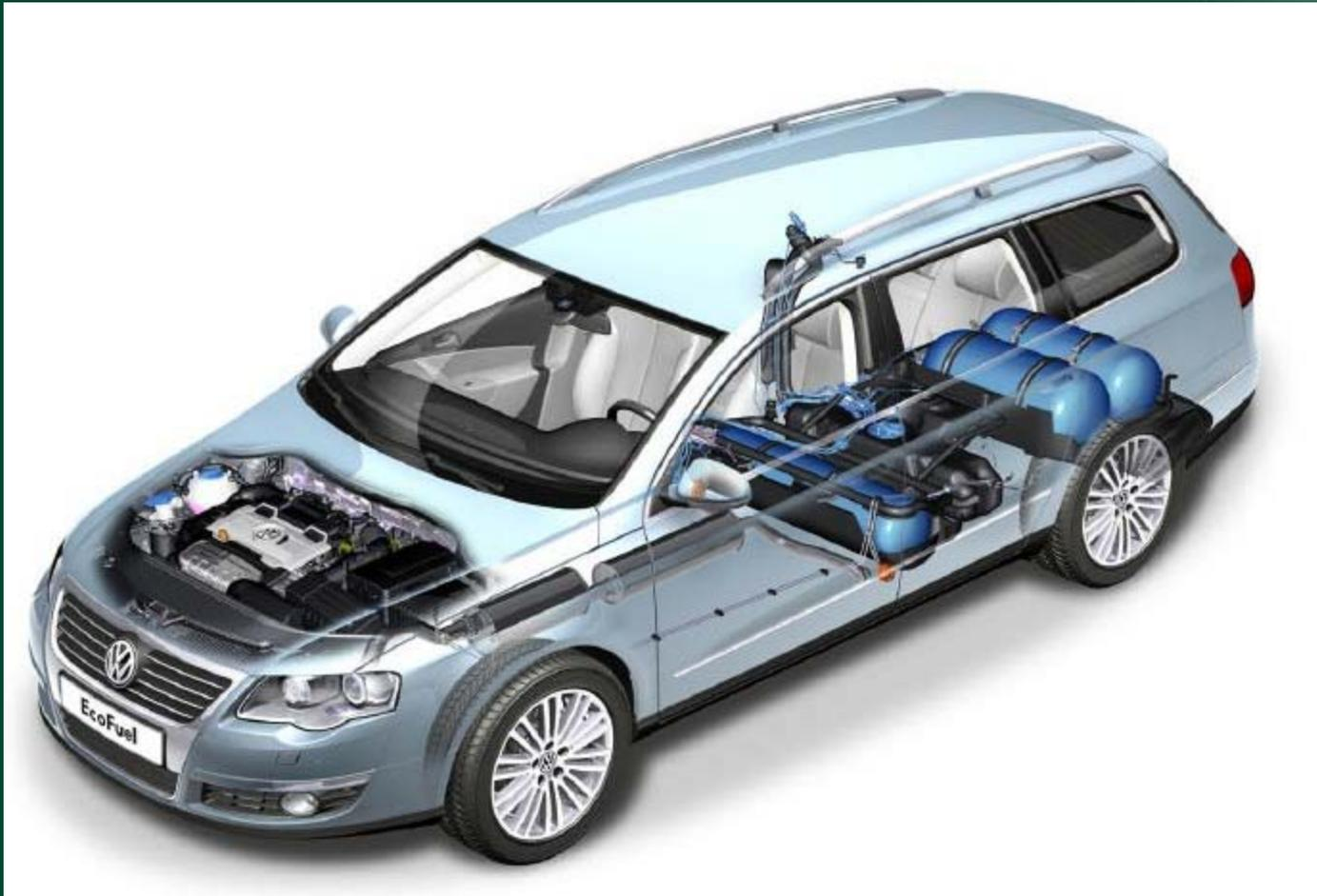
Dual Fuel CNG / Gasoline VW Passat
