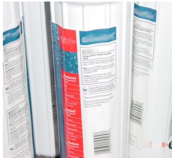
Figure 7. Examples of filters used for asbestos removal in the array in Figure 6. Photo courtesy of John Pavitt, USEPA Region 10. No endorsement implied. Information included for instructional purposes only.
