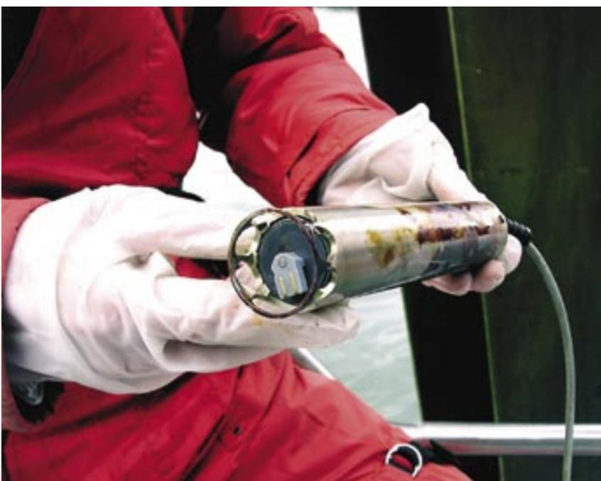
Water quality monitoring devices similar to this automatically record temperature, dissolved oxygen, turbidity, specific conductivity, and chlorophyll content. USGS technicians are using the devices at six lower Columbia River sites as part of the Estuary Partnership water quality monitoring program.
