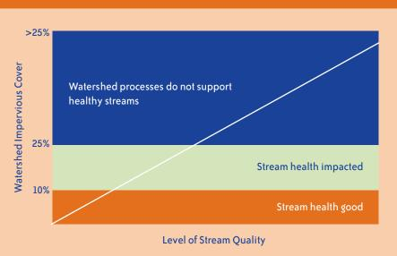
As impervious surface levels in a watershed increase, they typically correlate with a corresponding downward trend in stream quality.
