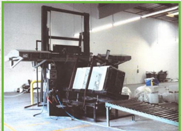
Refrigerator band saw. Photo by Michael Dunham. Image courtesy of JACO Environmental. © JACO Environmental
