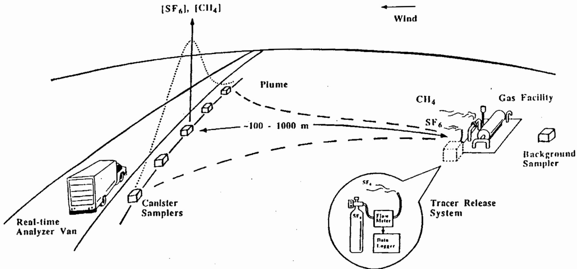
Figure 5-1. Schematic of the Tracer Ratio Emission Measurement Method
