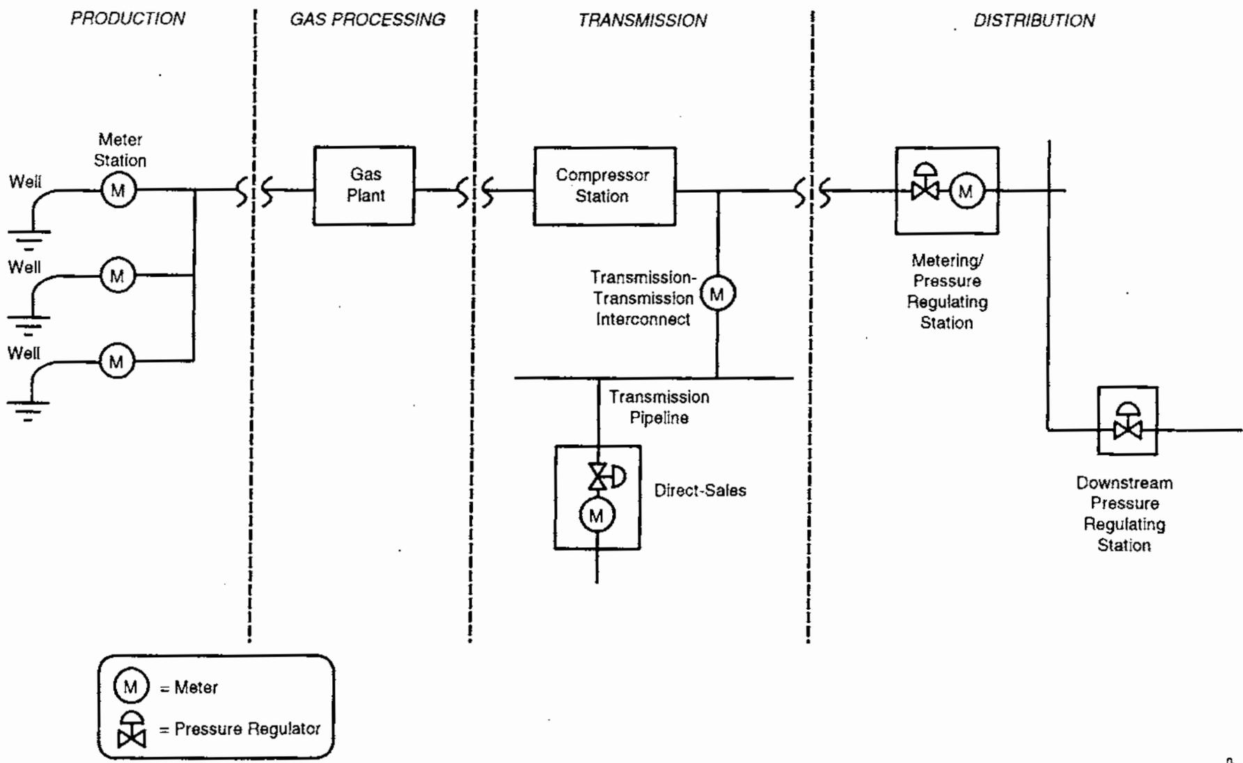
Figure 3-1. Metering/Pressure Regulating Facilities in the Gas Industry
