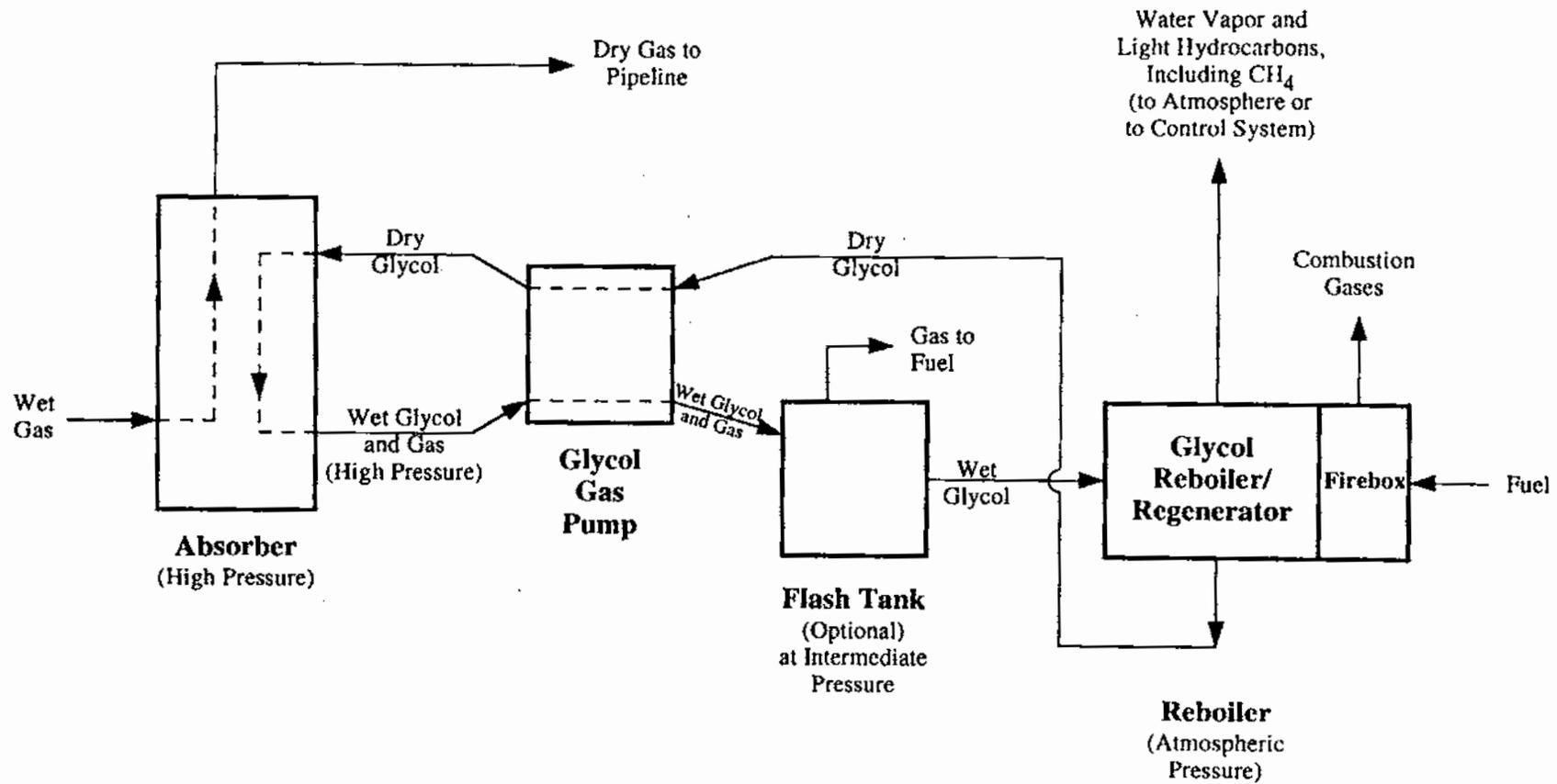
Figure 3-1. Block Process Flow Diagram of a Typical Glycol Dehydrator
