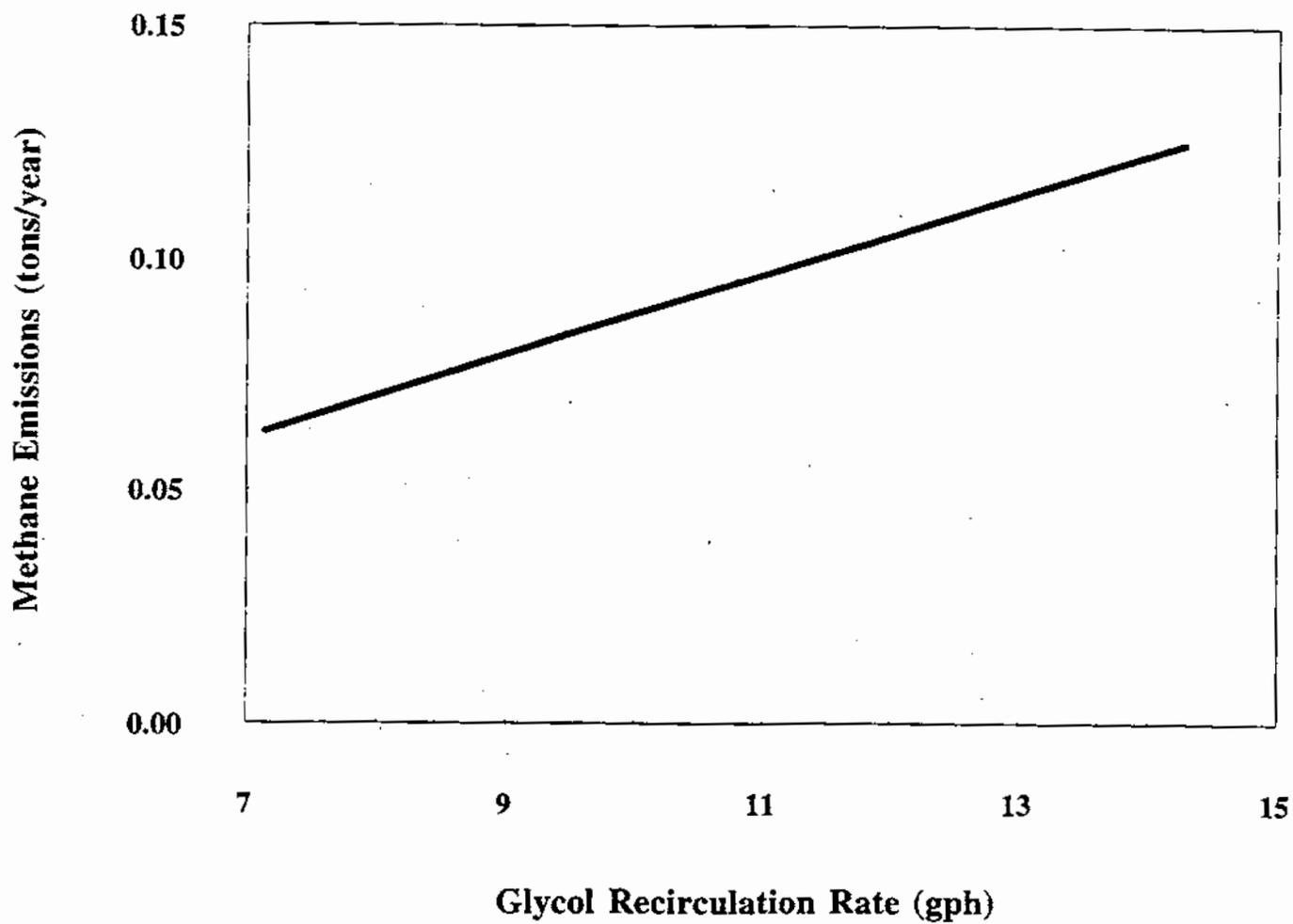
Figure 5-2. Methane Emissions - Glycol Regenerator Effect on Glycol Recirculation Rate
