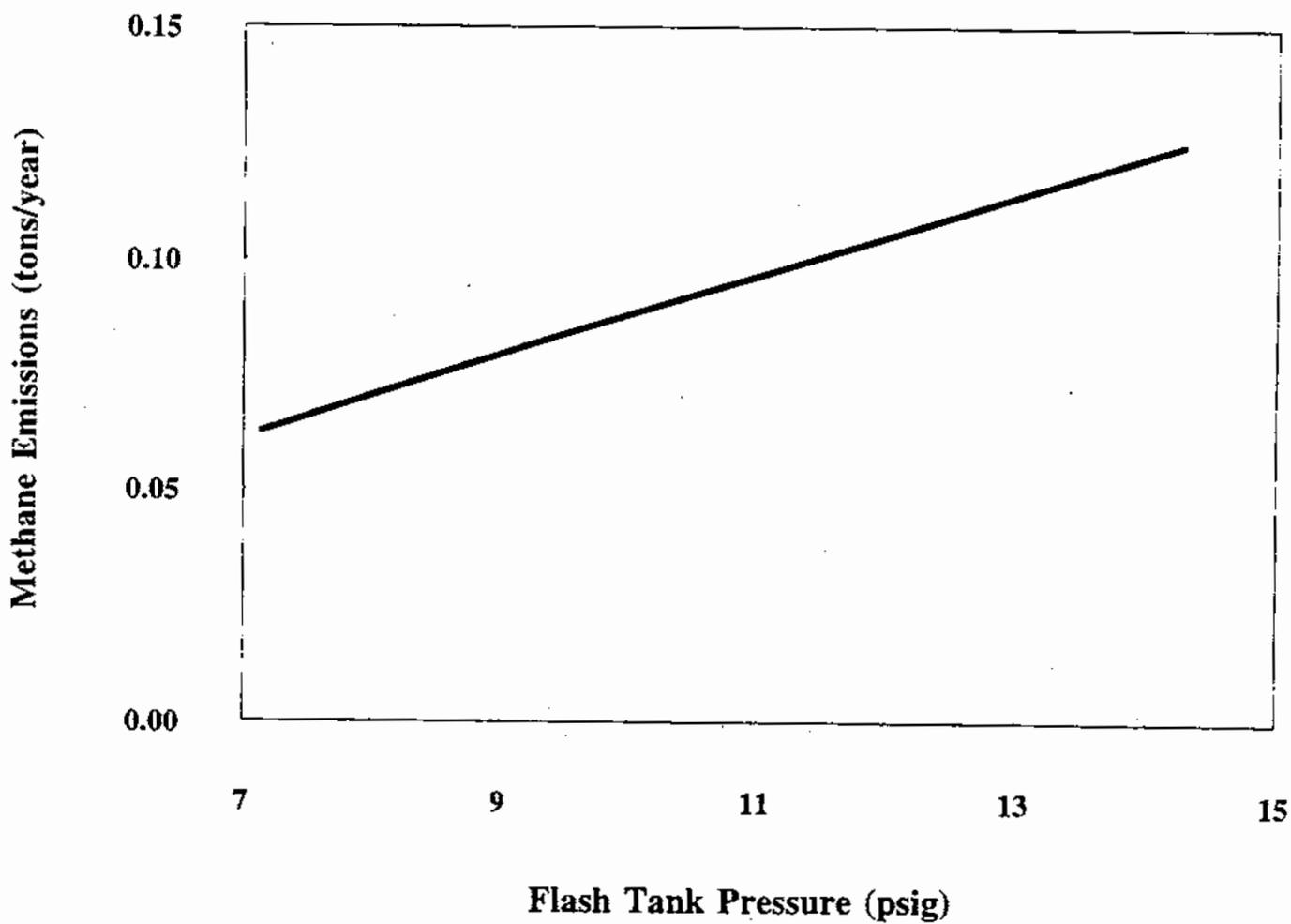
Figure 5-3. Methane Emissions - Glycol Regenerator Effect on Flash Tank Pressure
