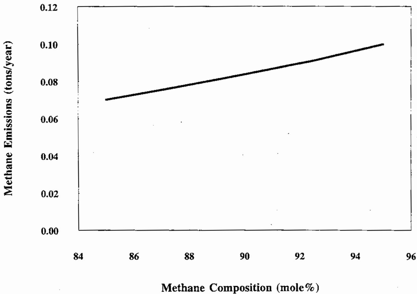
Figure 5-1. Methane Emissions - Glycol Regenerator Effect on Methane Composition
