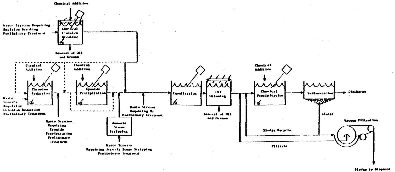
FIGURE 3-5. PSES/PSNS OPTION 1 AND 2 TREATMENT TRAIN FOR THE NONFERROUS METALS FORMING AND METAL POWDERS CATEGORY
