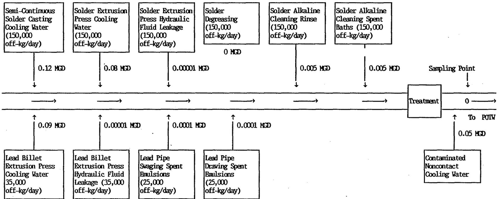
FIGURE 5-3. PROCESS FLOW DIAGRAM FOR A LEAD PIPE FORMING FACILITY
