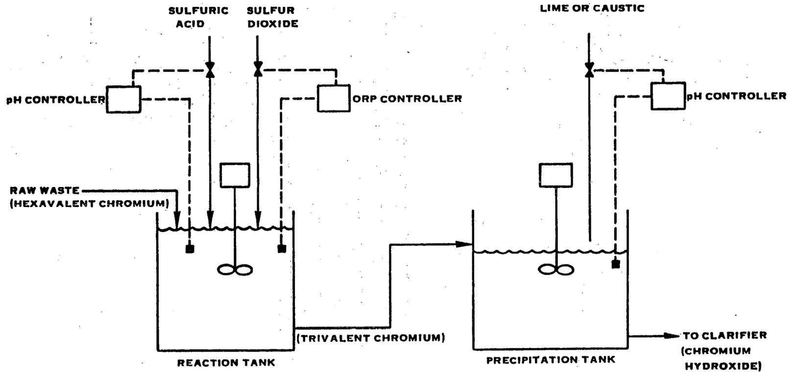
FIGURE VII-13. HEXAVALENT CHROMIUM REDUCTION WITH SULFUR DIOXIDE
