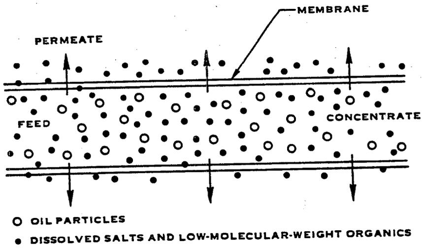
FIGURE VII-29. SIMPLIFIED ULTRAFILTRATION FLOW SCHEMATIC
