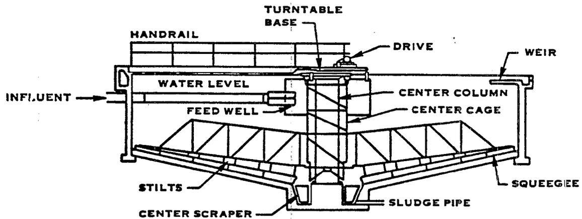
FIGURE VII-24. GRAVITY THICKENING
