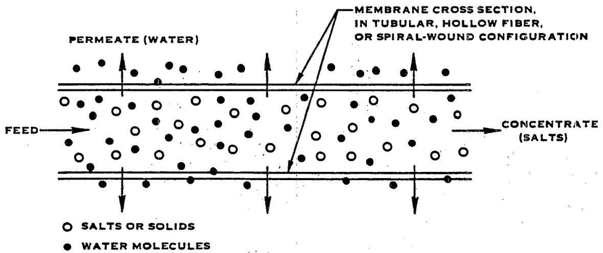
FIGURE VII-26. SIMPLIFIED REVERSE OSMOSIS SCHEMATIC
