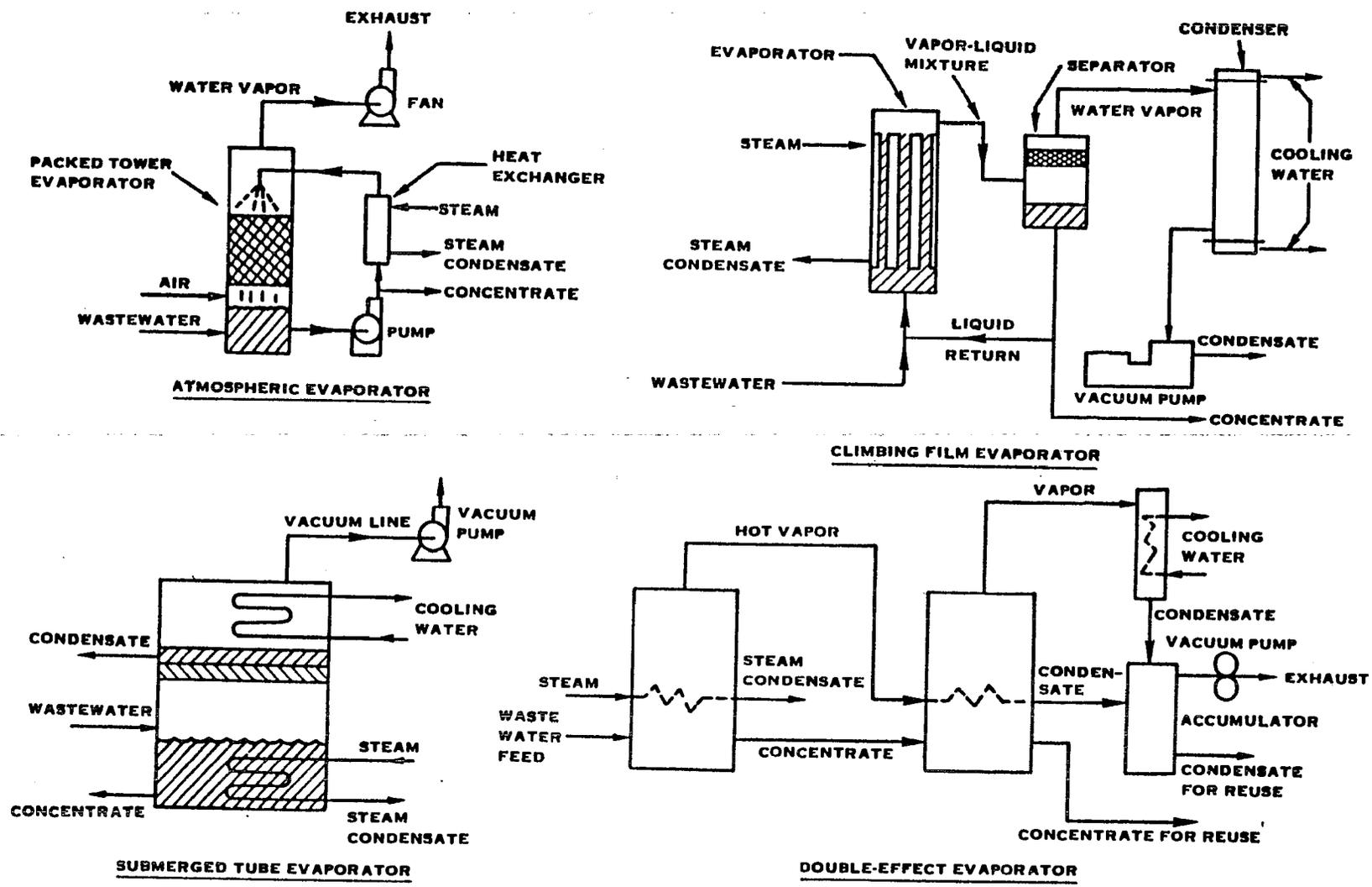
FIGURE VII-22. TYPES OF EVAPORATION EQUIPMENT
