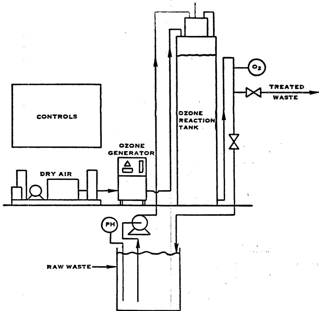
FIGURE VII-20. TYPICAL OZONE PLANT FOR WASTE TREATMENT
