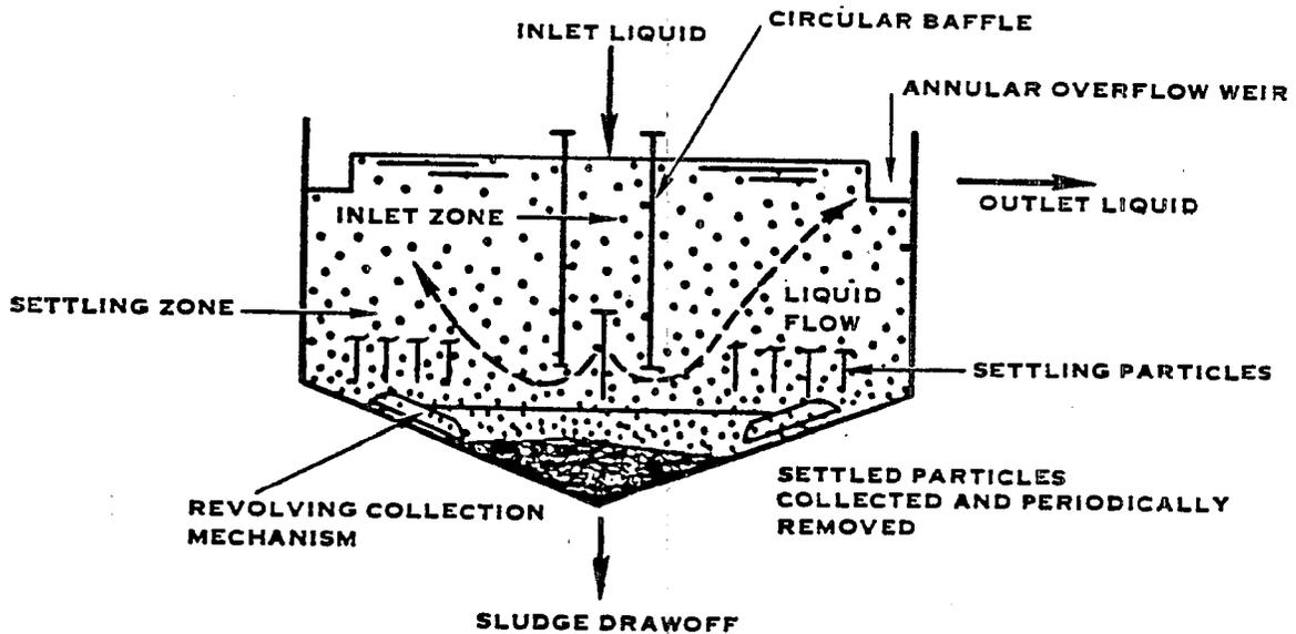
**FIGURE VII-16. REPRESENTATIVE TYPES OF SEDIMENTATION**
