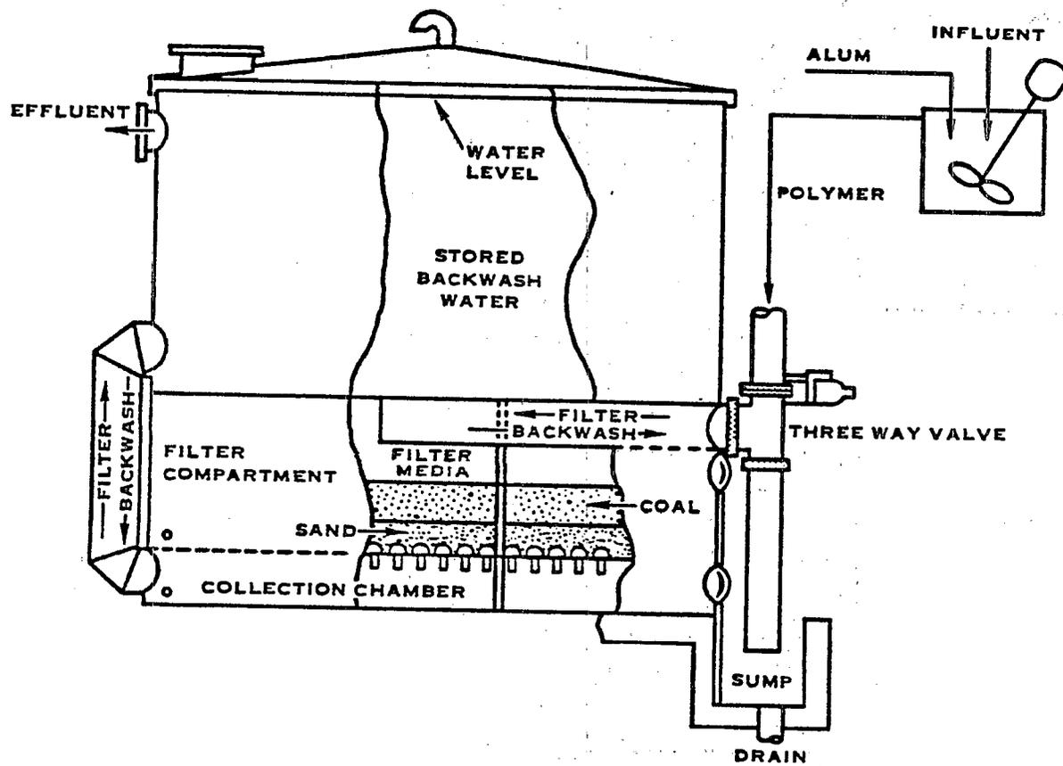
FIGURE VII-14. GRANULAR BED FILTRATION
