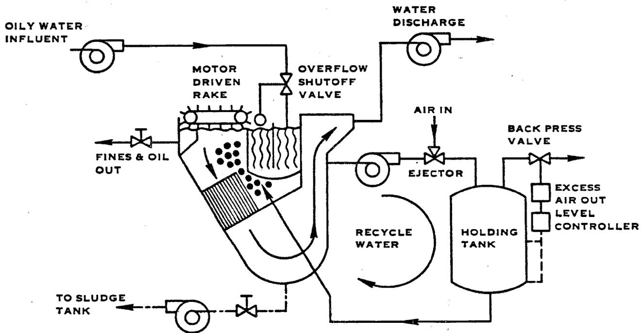
FIGURE VII-23. DISSOLVED AIR FLOTATION
