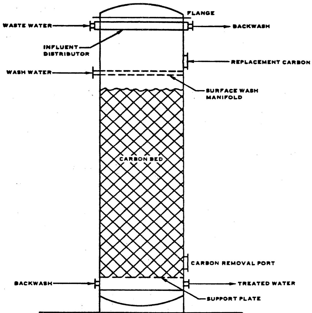
**FIGURE VII-17. ACTIVATED CARBON ADSORPTION COLUMN**
