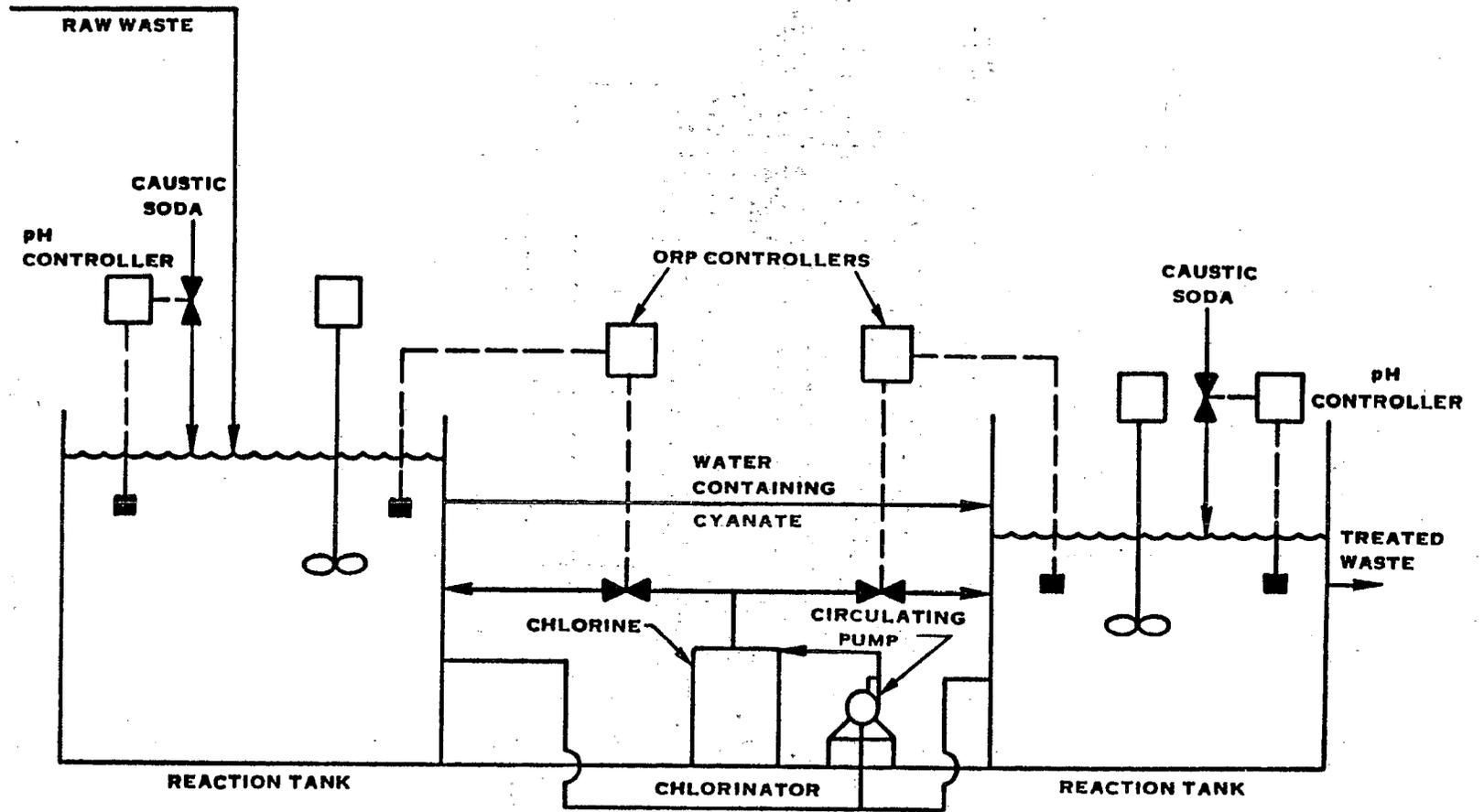
FIGURE VII-19. TREATMENT OF CYANIDE WASTE BY ALKALINE CHLORINATION
